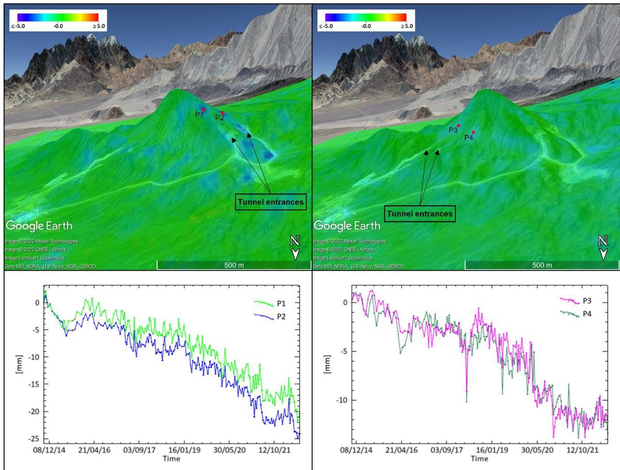
FIG. 3. Descending (left) and ascending (right) SBAS, Sentinel-1, 2014-2022; overlaid on Planet Labs image from 19 August 2022, © 2022 Planet Labs. All rights reserved. Reprinted by permission; draped over Google Earth's terrain model.
