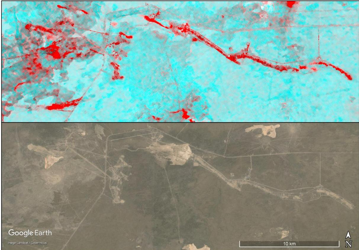
FIG. 1. Multitemporal coherence over West Mynkuduk ISL mining site, Sentinel-1, July 2021–July 2022, coefficient of variation in red, mean in blue (top); Google Earth/Image Landsat/Copernicus, December 2020 (bottom)
