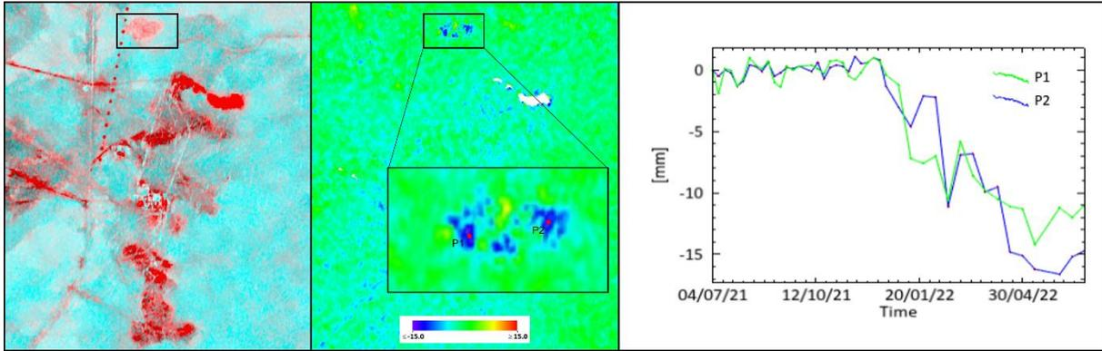
FIG. 2. Multitemporal coherence over West Mynkuduk ISL mining site, Sentinel-1, July 2021–July 2022, coefficient of variation in red, mean in blue (left); SBAS, Sentinel-1, July 2021–July 2022 (right)
