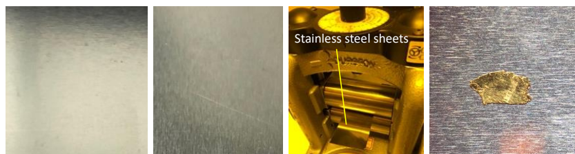
Figure 2. Mechanical alloying method using a hand-operated rolling mill. From left to right, photographs show the gold foil after source deposition, after folding, the rolling mill with the gold foil sample sandwiched by stainless steel sheets for preventing contamination, and the rolled-out gold foil as a result.
