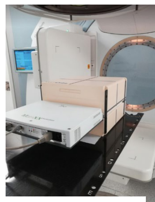
Figure 2. Setup of phantom for planar dose measurement
