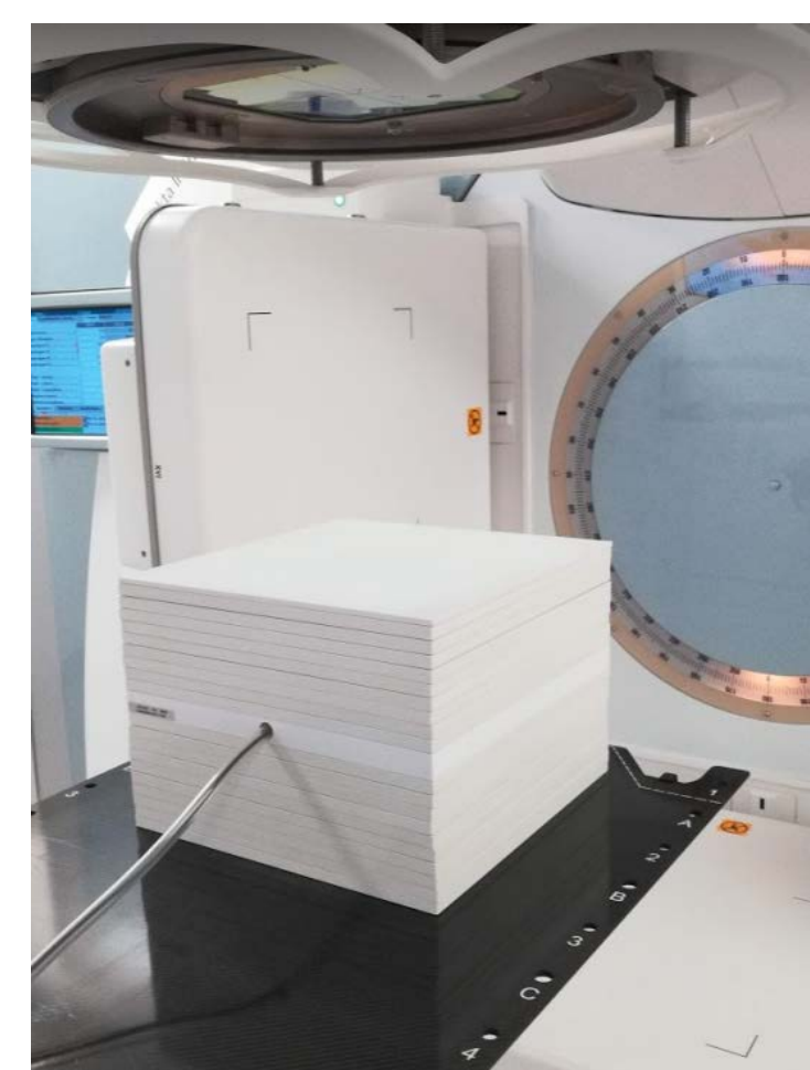
Fig1. Setup of phantom for 1point dose measurement
