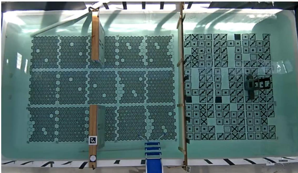
FIG. 2. The pool showing the two simulated spent fuel ponds and some of the obstacles.
