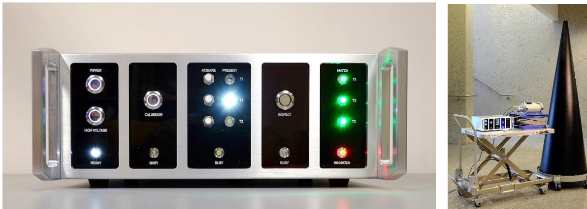
FIG. 1. Information Barrier Experimental (IBX). Front panel and user interface (left), experimental setup with mock-up warhead (right).
