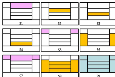
FIG. 2. Schematic representation of various scenarios: light violet refers to sodium plenum zones, amber to fuel zones; figure taken from [10].
