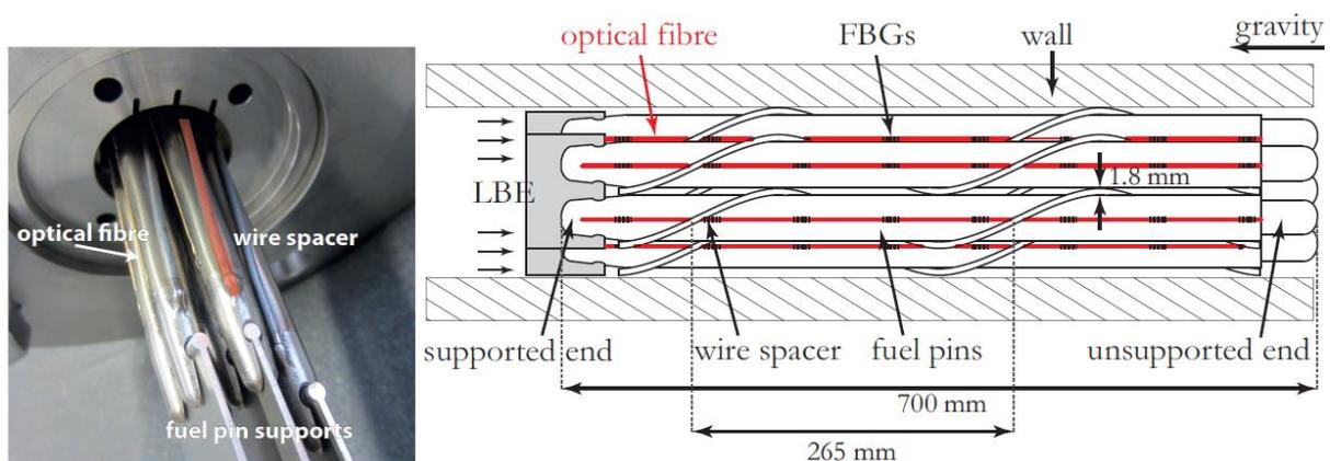
FIG. 6. Seven-pin, reduced-length FA instrumented for flow-induced vibrations at SCK•CEN [16]
