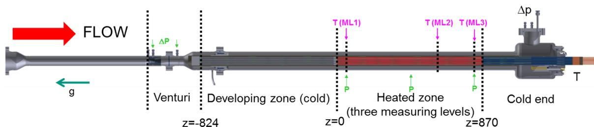
FIG. 2. Side view of the heated 19-rod bundle test section at KIT, indicating the instrumentation [9]
