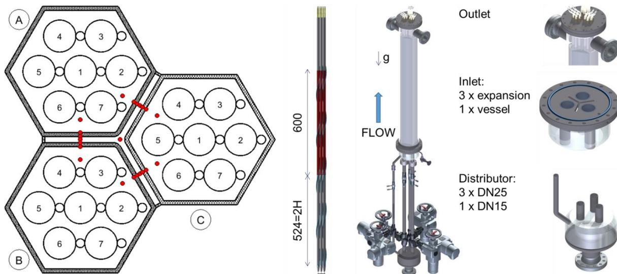
FIG. 7. Inter-wrapper flow test section with three 7-rod bundles at KIT
