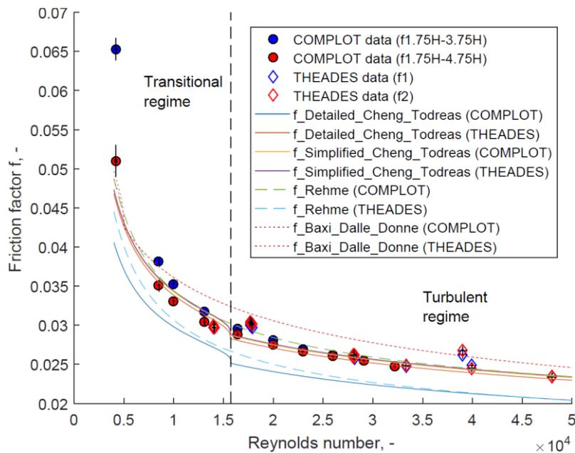
FIG. 1. Measured and predicted pressure drop across the 127-pin MYRRHA fuel bundle
