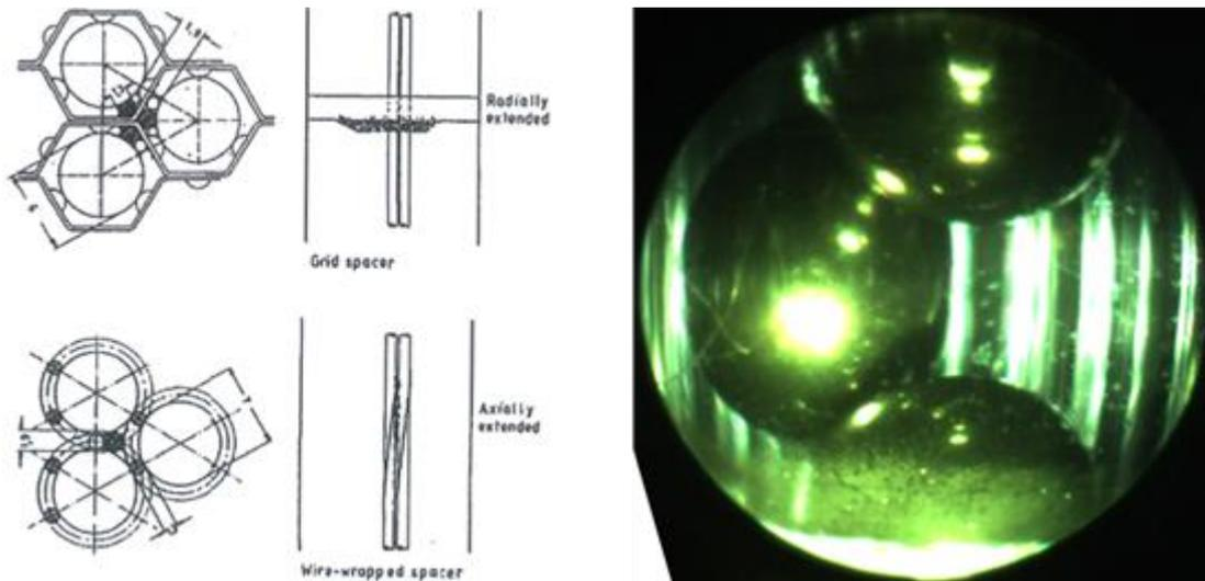
FIG. 5. Process of blockage formation and growth by accumulation of particles. Left: effect of grid and wire spacers [15]. Right: preliminary results of optical instrumentation at KIT
