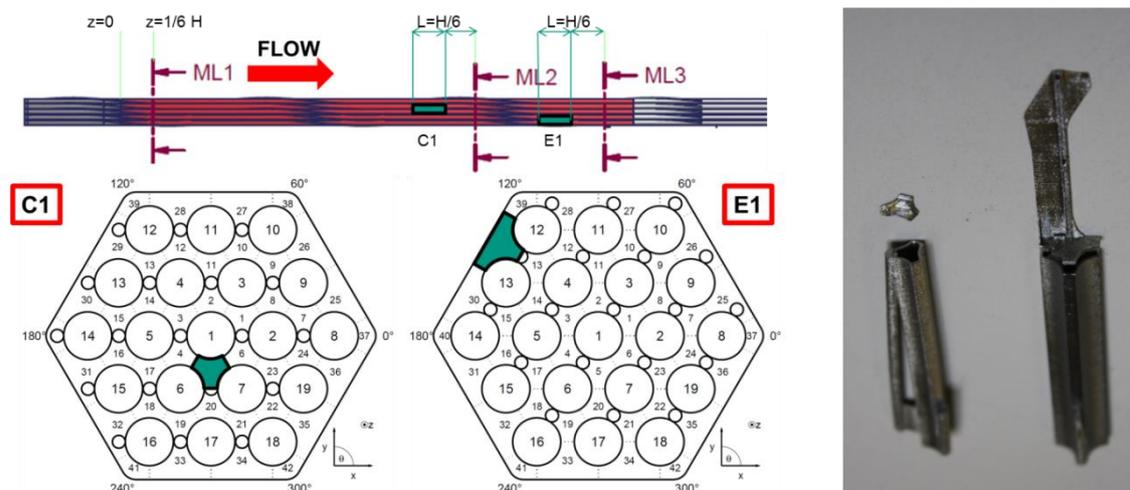
FIG. 4. Local flow blockages in a 19-rod bundle studied at KIT in the MAXSIMA project [14]
