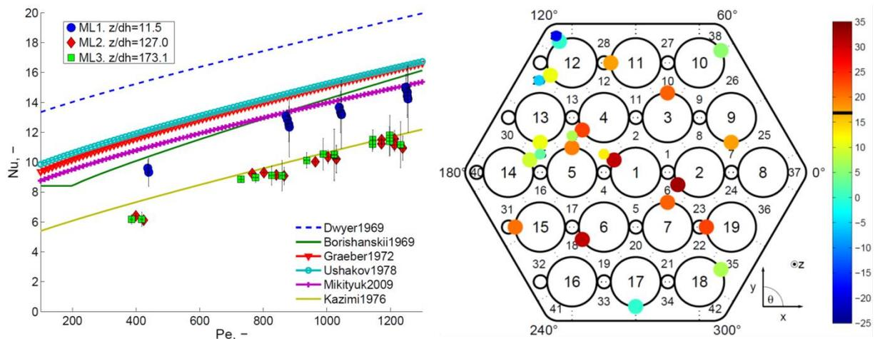
FIG. 3. Experimental heat transfer results in a 19-rod bundle. Left: Nusselt number, compared to several correlations. Right: local temperature above bulk ( $T-T_b$ ) for a reference case [9]
