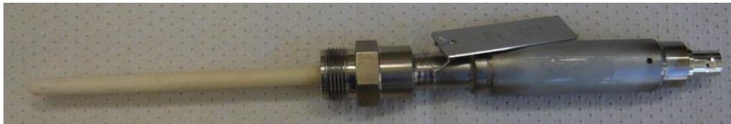
FIG. 6. Oxygen sensor fabricated by JAEA
