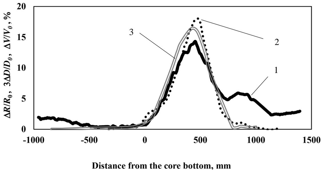
FIG. 1. Relative variation of electrical resistivity  $\Delta R/R_0$  (1), diameter  $3\Delta D/D_0$  (2) and swelling  $\Delta V/V_0$  (3) changes for BN-600 cladding specimens.
