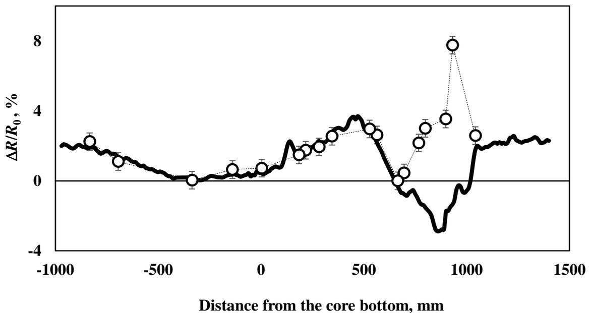
FIG. 4. Resistograph image of the fuel element with EK-164 cladding (—) and relative electrical resistivity of specimens of the dismantled fuel element (○).
