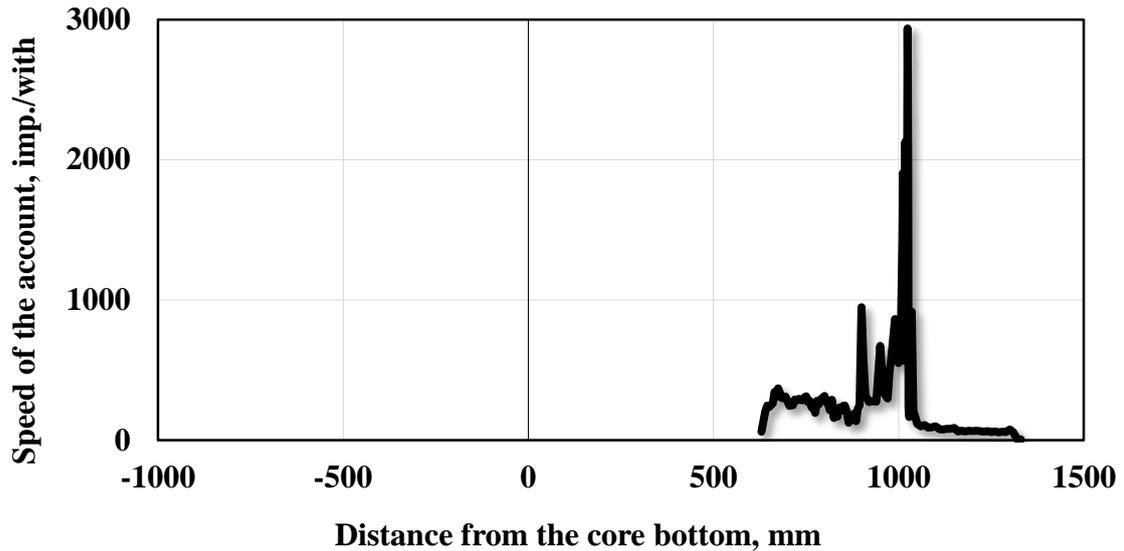
FIG. 3. Fission product ( $^{137}\text{Cs}$ ) distribution along the fuel element according to gamma spectrometry data.
