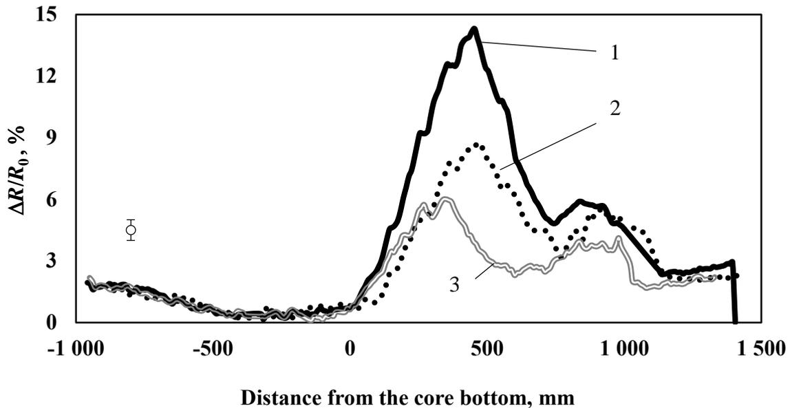
FIG. 2. Electrical resistivity value for ChS-68 cladding material at damage doses of 83 (1), 71 (2) and 58 (3) dpa.
