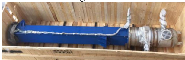
FIG. 3. CLEAR-S main heat exchanger.
