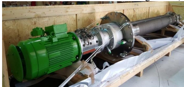
FIG. 2. CLEAR-S Primary loop pump.
