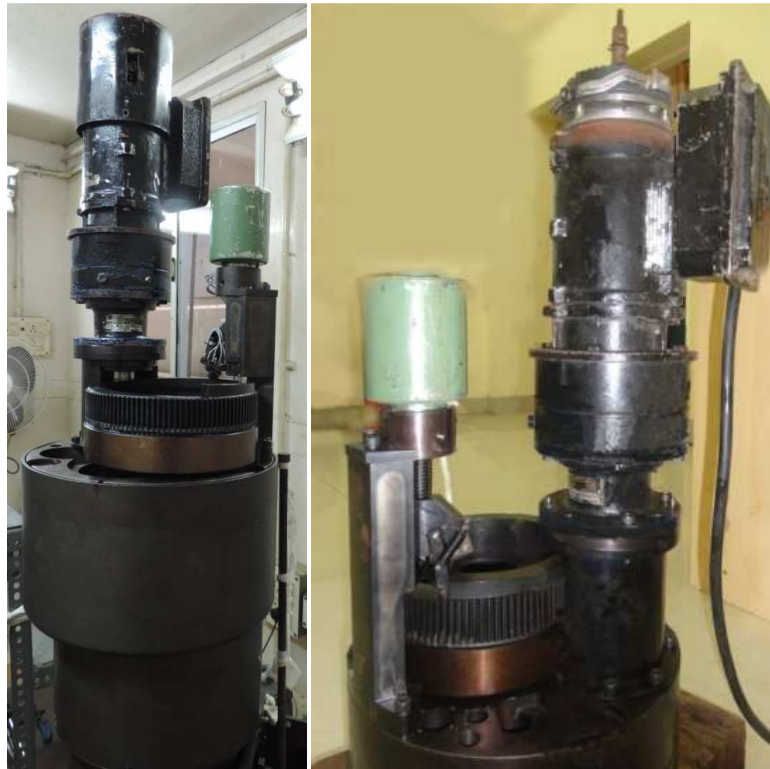
Figure 5: Photograph of Stroke limiting device integrated with CSRDM left & SLD unit- right
