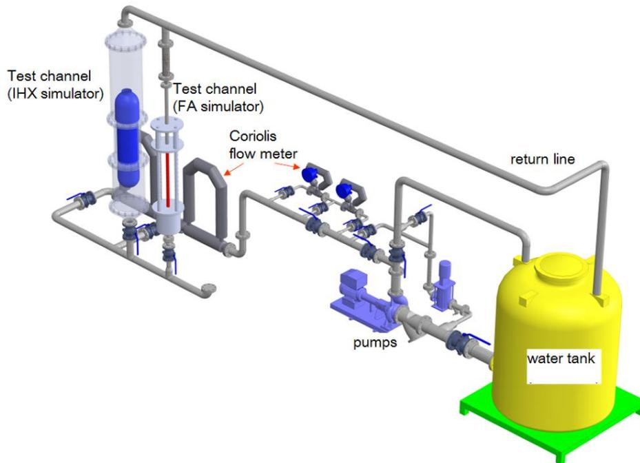
FIG. 11. CALIP loop for calibration
