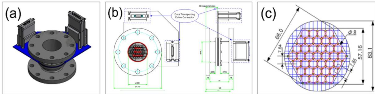
FIG. 5. Design of a wire mesh sensor for 37-rod assembly
