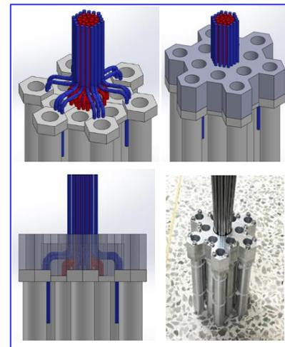
FIG. 9. Assembling of pressure impulse line
