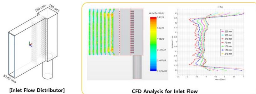
*FIG. 14. IHX inlet flow distributor design and CFD validation*
