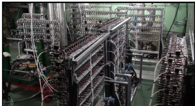
FIG. 12. (a) Schematics and (b) photograph of solenoid valve network
