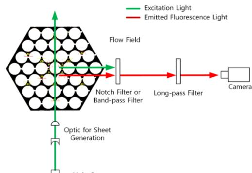
FIG. 6. Schematic diagram for LIF experiment
