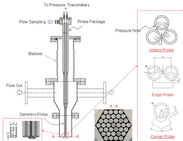
FIG. 4. Iso-kinetic sampling probe and installation
