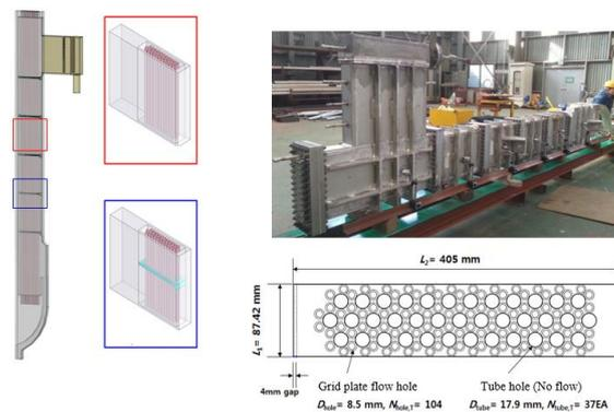
FIG. 13. IHX Test Facility Design
