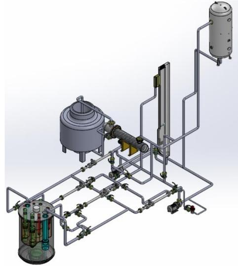
*FIG 15 Schematic of reactor flow and IHX flow characteristics test loop*
