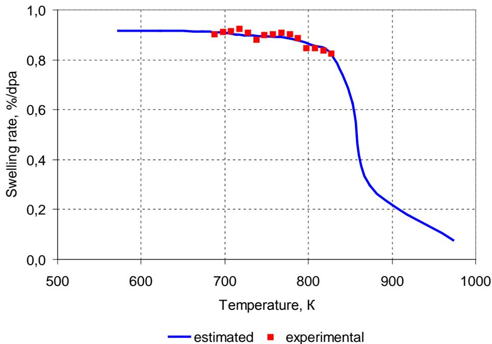
FIG. 7. Irradiation temperature dependence of dose swelling rate of ChS-68 steel for displacement rate of  $1 \times 10^{-6}$  dpa/s [10].
