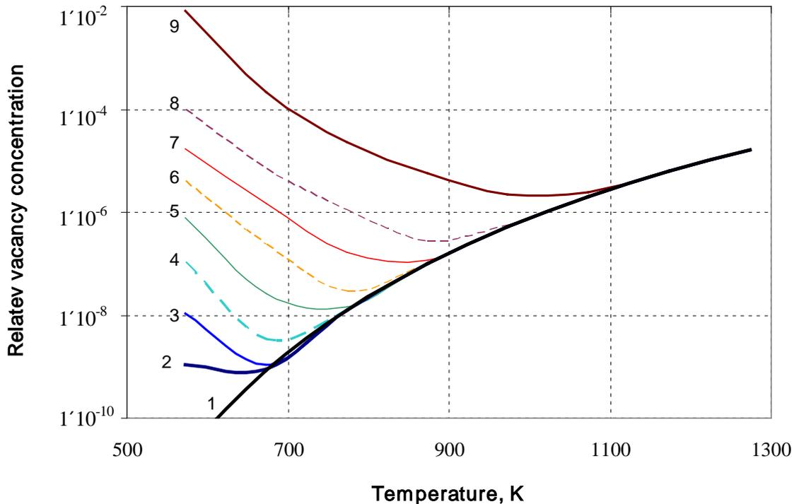
FIG. 1. Irradiation temperature dependence of steady-state vacancy concentration in ChS-68 steel at different displacement rates: 1 – thermally equilibrium concentration, 2 –  $10^{-10}$  dpa/s, 3 –  $10^{-9}$  dpa/s, 4 –  $10^{-8}$  dpa/s, 5 –  $10^{-7}$  dpa/s, 6 –  $10^{-6}$  dpa/s, 7 –  $10^{-5}$  dpa/s, 8 –  $10^{-4}$  dpa/s, 9 –  $10^{-2}$  dpa/s.
