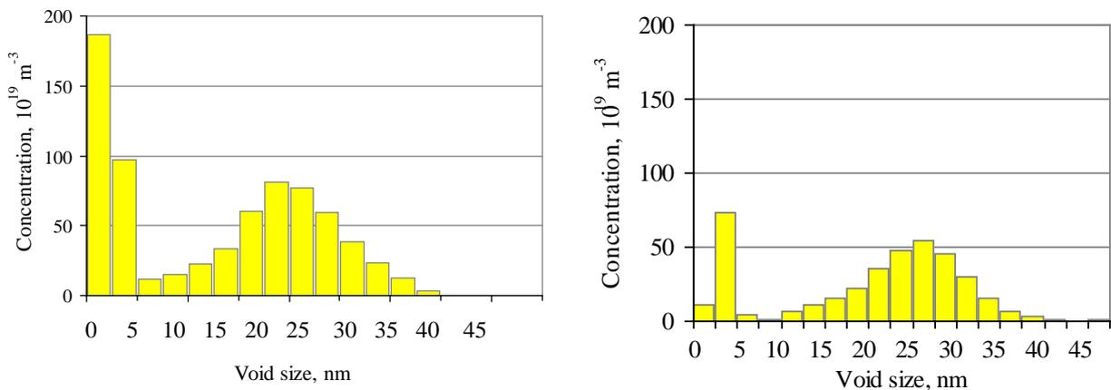
FIG. 4. Bar chart of void distribution in cladding specimens from areas of low-temperature irradiation  $443 \pm 3 \text{ }^\circ\text{C}$  ( $716 \pm 3 \text{ K}$ ):
