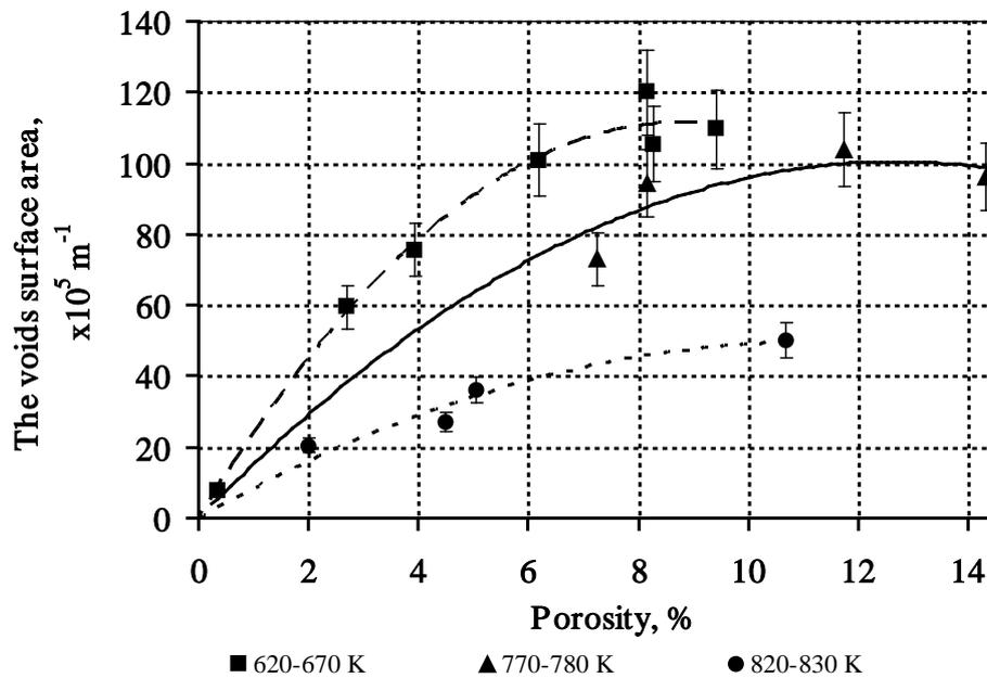
FIG. 5. Dependence of integral area of void surface on porosity value in ChS-68 steel at different irradiation temperatures in the range between 410 and 560 °C.
