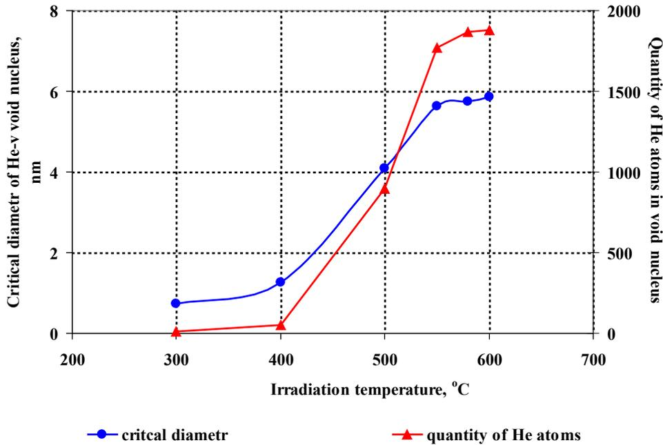
FIG. 3. Irradiation temperature dependence of critical diameter of helium-vacancy void nucleus and helium concentration in it [6].
