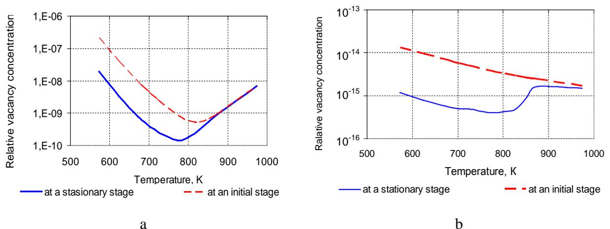
FIG. 6. Irradiation temperature dependence of point defect concentration in ChS-68 steel at the steady-state swelling and initial stages: a – for vacancies; b – for interstitial atoms [10].
