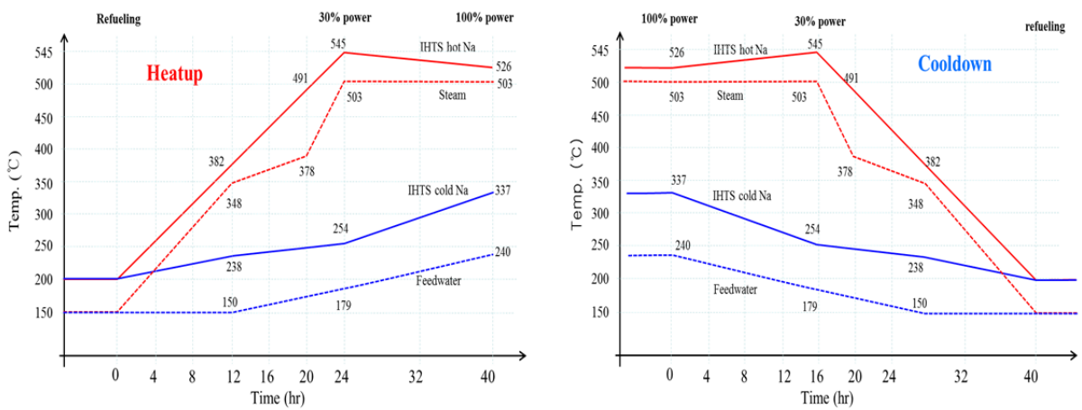
(a) Time histories of fluid temperature for heatup and cooldown operations
