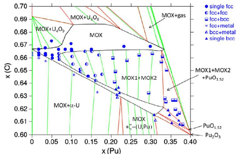
Figure 1 : Calculated phase diagram of the U-Pu-O system
