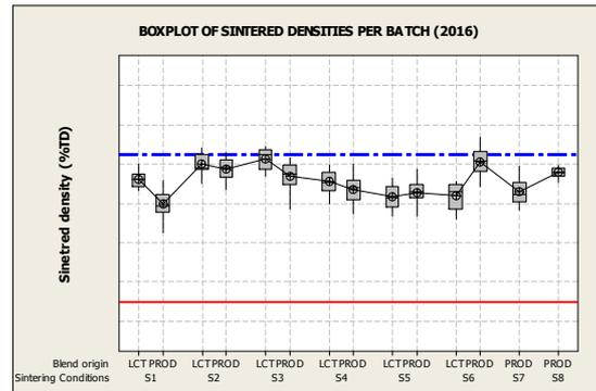
*Fig. 8: Calculated sintered densities population per batch*
