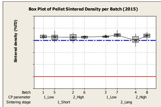
*Fig. 4: Calculated sintered densities population vs sintering parameter and compression pressure*
