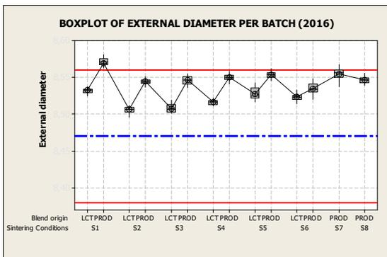
Fig. 5: External sintered diameters population per batch
