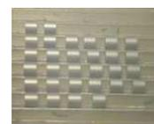
Sintered pellets on tray for visual inspection
