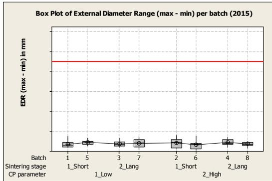
*Fig. 3: EDR population vs sintering parameter and compression pressure*
