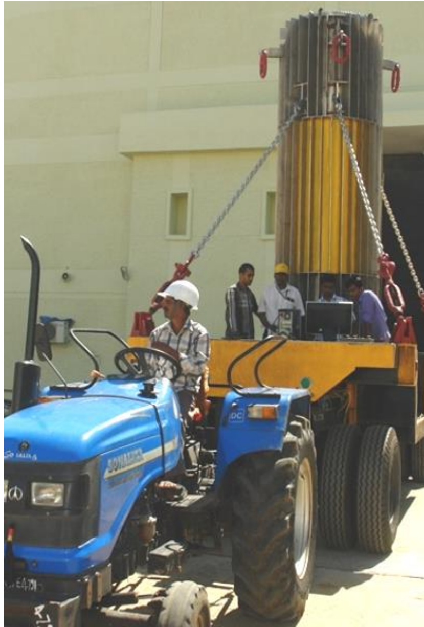
FIG. 1. Photograph for the mockup trial transportation arrangement for the dummy fuel subassembly.
