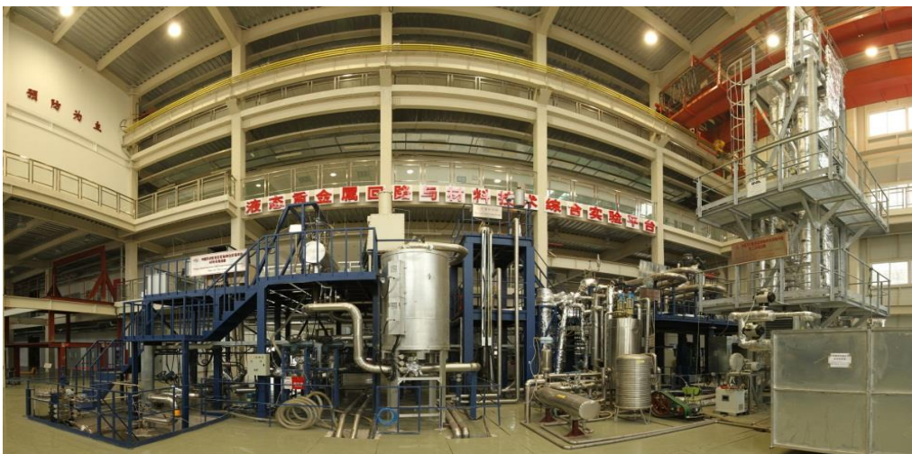
FIG. 3. Multi-functional lead-bismuth loop KYLIN-II.
