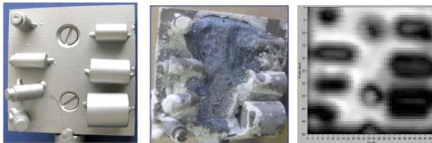
FIG. 9 Joyo-pin target sample before and after sodium tests and intensity image of the target sample at 177°C and FD = 25.4mm.
