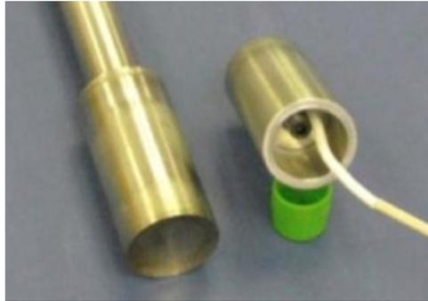
FIG. 3. High-temperature submersible PZT-5A prototypes: (left) prototype #1 after complete sealing and (right) prototype #2 before sealing
