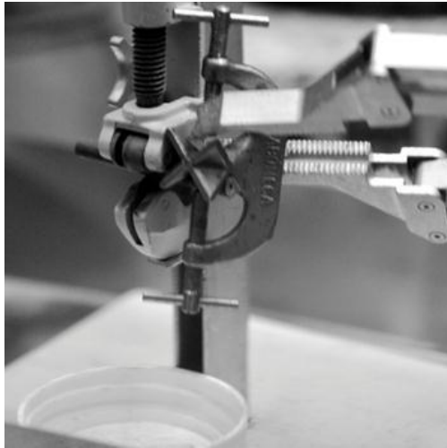
FIG. 4. Fuel cutting with tube cutter
