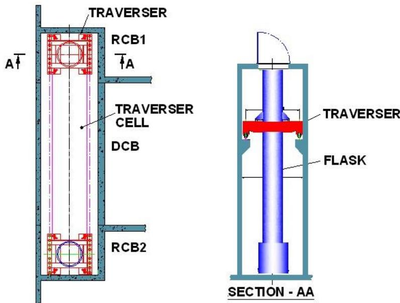
FIG. 9. Traverser for Special Handling
