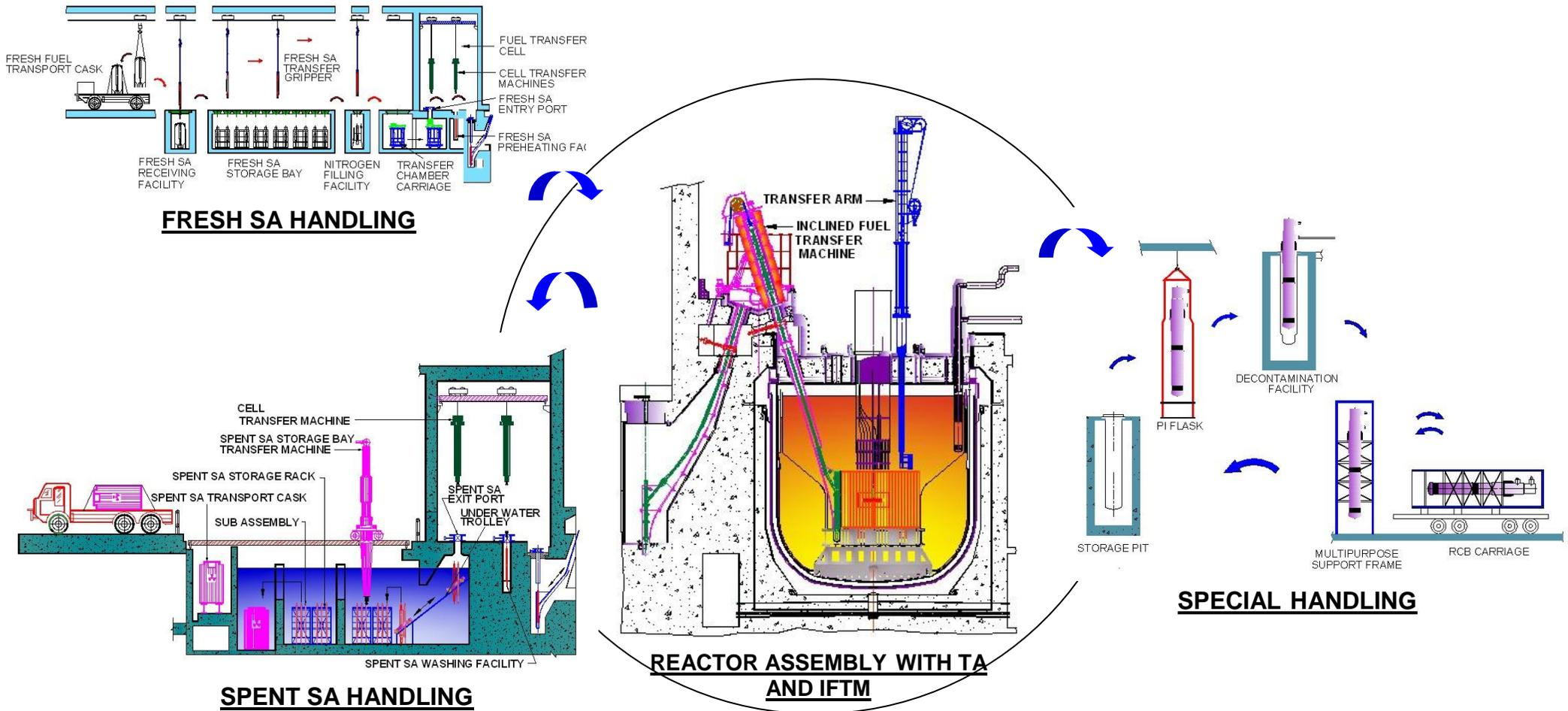
FIG. 2. Component Handling System in PFBR
