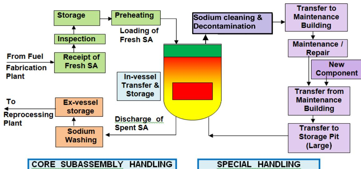
FIG.1. Sequence of Component Handling
