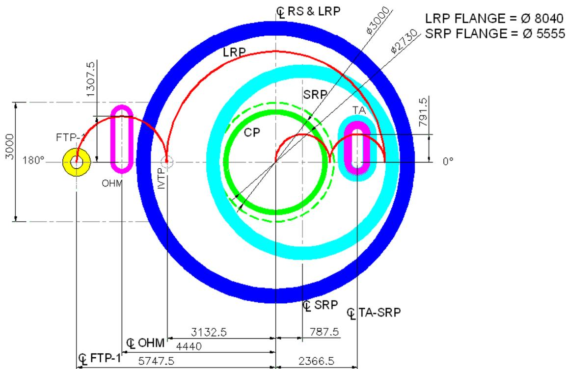
FIG. 6. In-Vessel Handling Scheme for FBR 1&2
