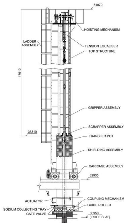
FIG. 7. Subassembly Transfer Flask
