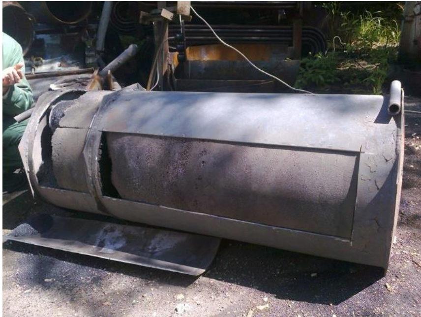
FIG. 4. Modernized RV with final product (70 liters of secondary sodium).
