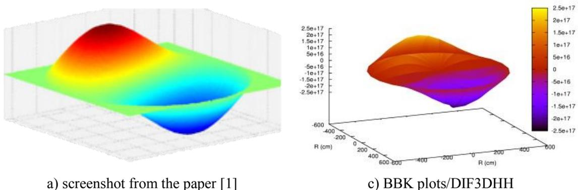
FIG. 3. Comparison of the radial distribution of the second harmonic neutron fluxes.
