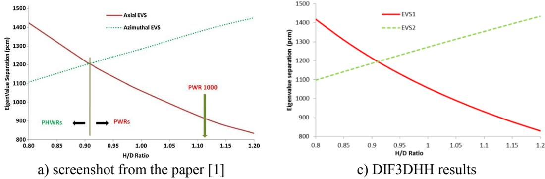
FIG. 4. Results of the effect of core shape.
