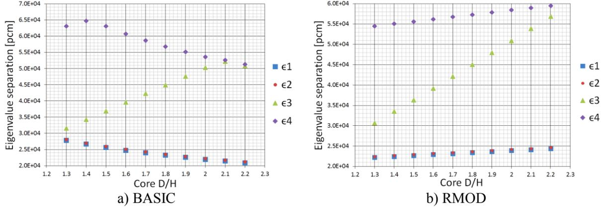
FIG. 6. Results of eigenvalue separations of the BASIC and RMOD approach.
