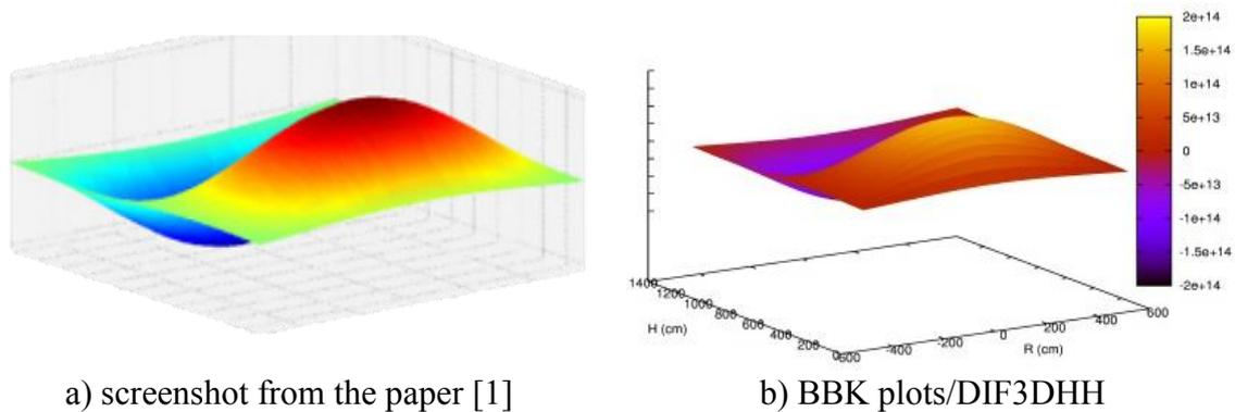
FIG. 2. Comparison of the axial distribution of the first harmonic neutron fluxes.
