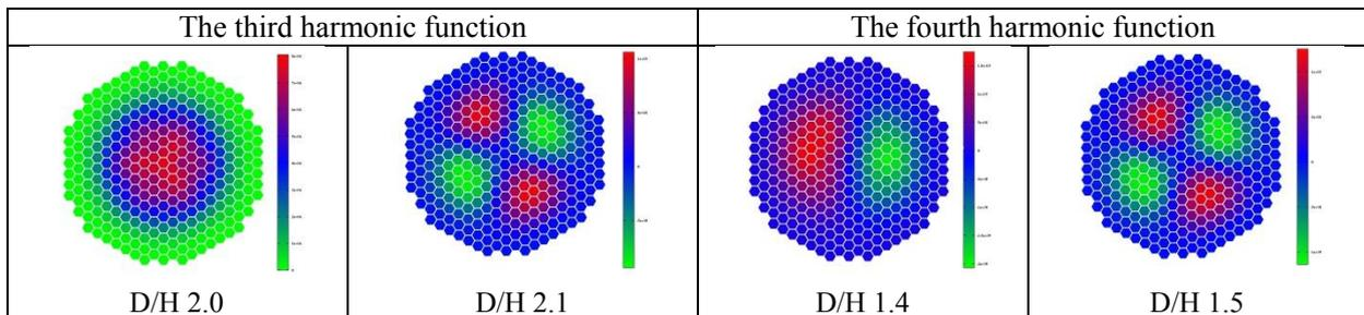
For D/H bellow 1.4 the radial distribution of the fourth harmonic neutron flux is similar to the first harmonic neutron flux. The core neutral line is almost perpendicular to the  $x$  axis, but a slight clockwise rotation can be observed. For D/H ratios above 1.5 there are two positive and two negative peaks of the neutron flux.
