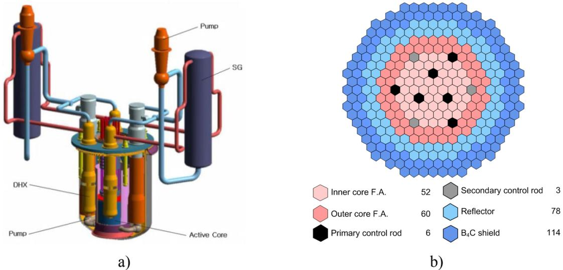
FIG. 1. The sketch and active core fuel loading pattern of PGSFR [9].
