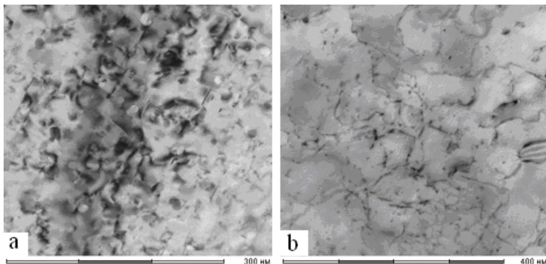
FIG. 7. Dislocation structure of the fuel pin cladding.
