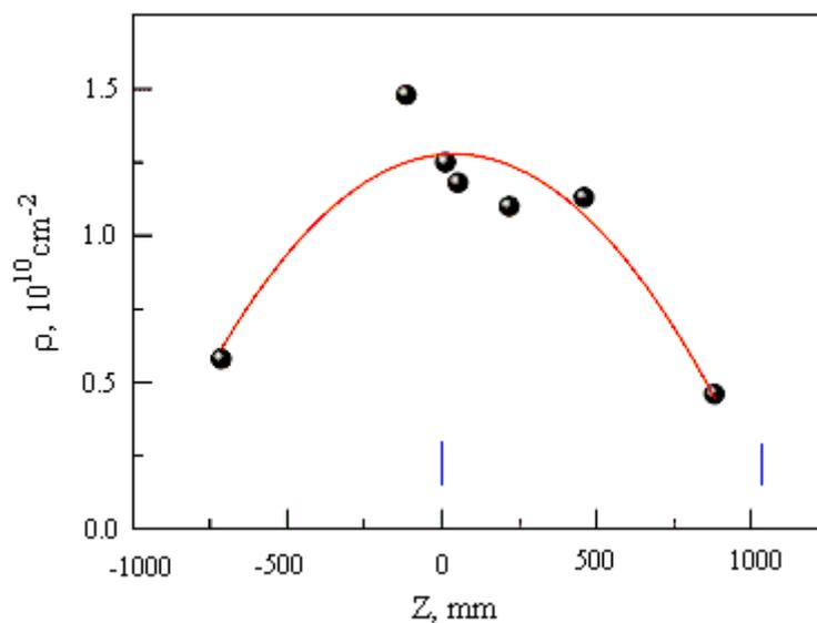
FIG. 5. Dislocation density as a function of the relative localization of samples in the reactor core (shown by blue vertical lines)
