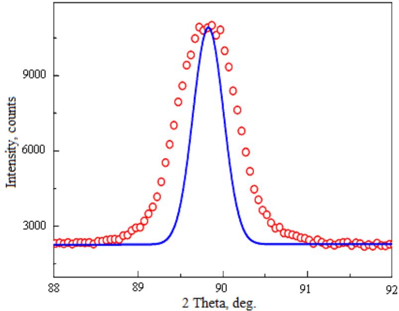
FIG.1. Experimental (circles) and reference (line) diffraction peak (311) for sample No 1.
