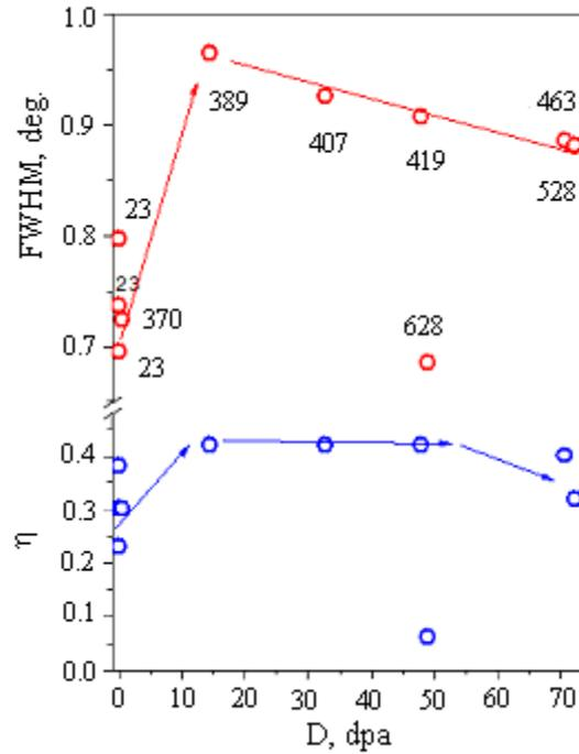
FIG.3. Dose dependences of the (311) peak width and coefficient  $\eta$  (relative fraction of Lorentzian in its form. Temperatures of irradiation are given in the panel near the circles. Temperature 23 C corresponds to not irradiated samples.
