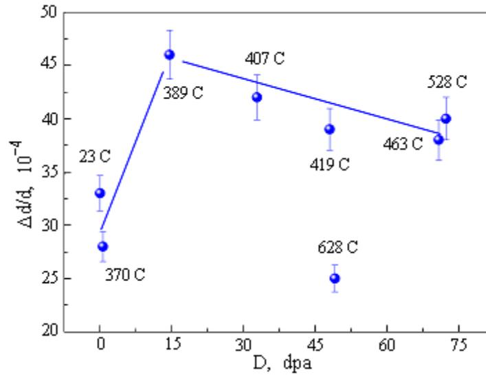
FIG. 4. Dependence of microdeformations averaged over directions for the samples of steel EK164 on irradiation dose. Temperatures of irradiation are given in the panel.
