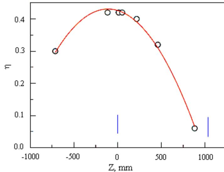
FIG. 6. Dependence of the coefficient of the reflection form  $\eta$  on the position of the sample in the core (designated by blue vertical lines)
