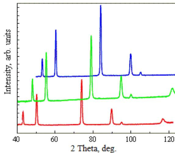
FIG. 2. Experimental neutron diffraction patterns for the samples prepared from the BN600 fuel pins: blue – initial state; green – the doze of 14.5 dpa at  $T=389^{\circ}\text{C}$ ; red – the doze of 72.3 at  $T=528^{\circ}\text{C}$ . For better illustration purposes, the patterns are shifted by the zero angle and height.
