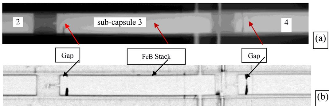
Fig. 5. Post-irradiation neutron radiograph (a) raw image (b) processed image
