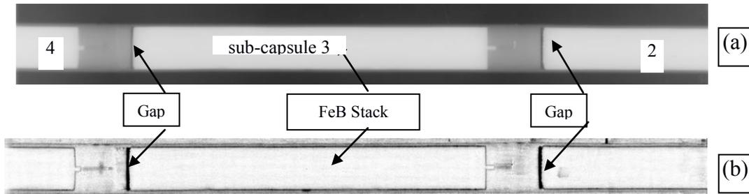
Fig. 4. Pre-irradiation neutron radiograph (a) raw image (b) processed image
