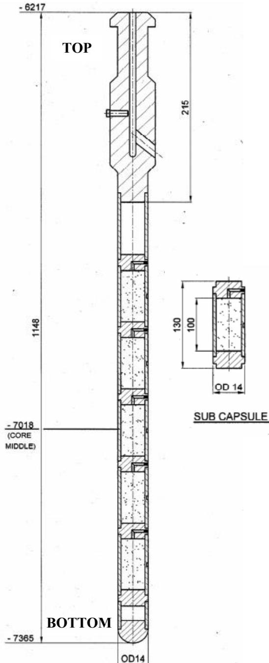
Fig. 1. Sketch of ferroboron irradiation capsule.
