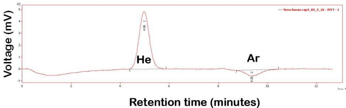
Fig 3: Chromatogram obtained during the analysis of gas extracted from one of the ferroboron sub-capsules.
