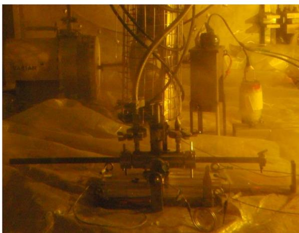
*Fig.2: Helium gas extraction set-up inside the hot cell*
