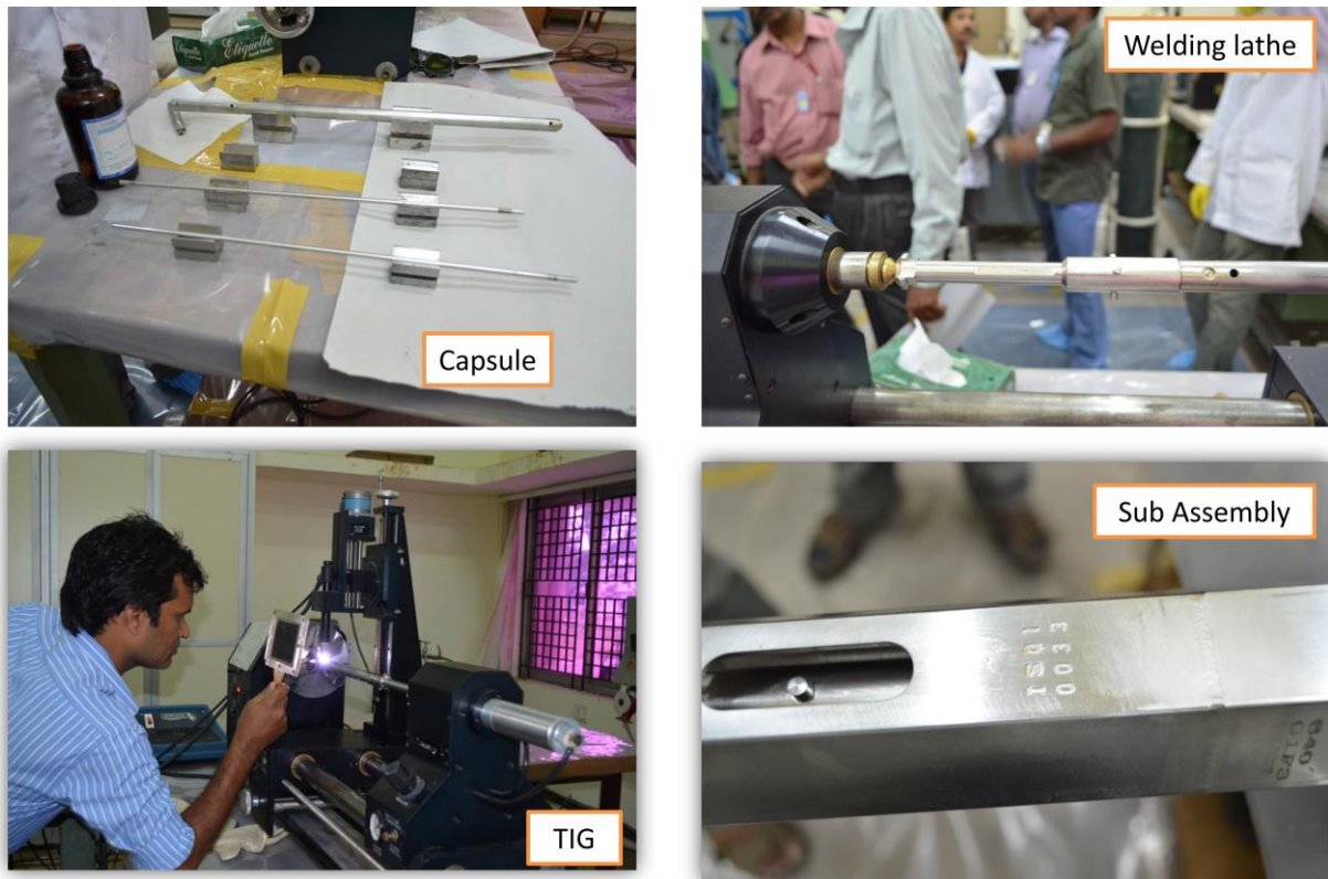
Fig. 10. Fabrication of irradiation capsule for test irradiation in FBTR
