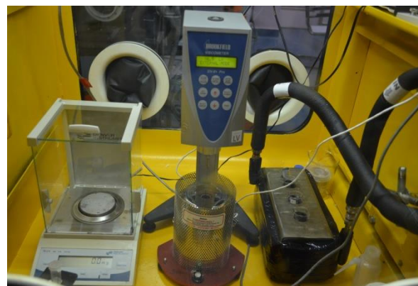
Fig. 12. Broth preparation and viscosity measurement inside another part of the glove box
