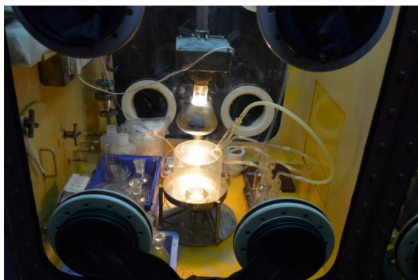
Fig. 11. The plutonium nitrate preparation inside part of a glove box
