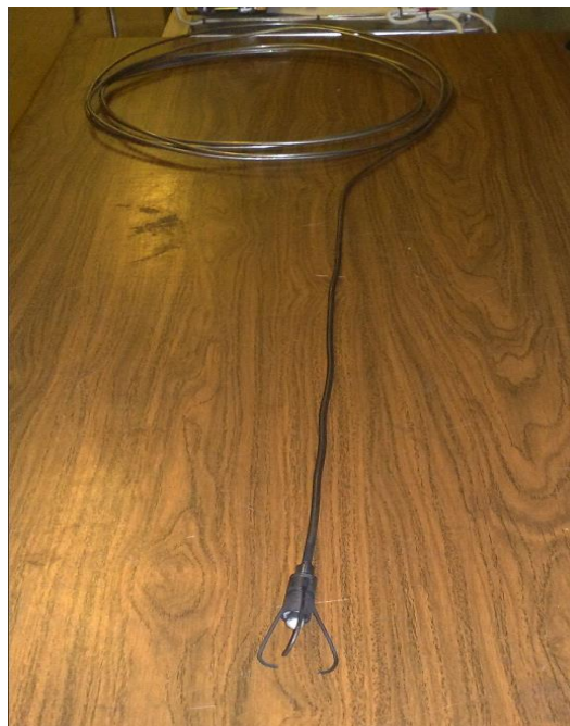
Figure 3 – Oxygen activity sensor with a length of 8 m
