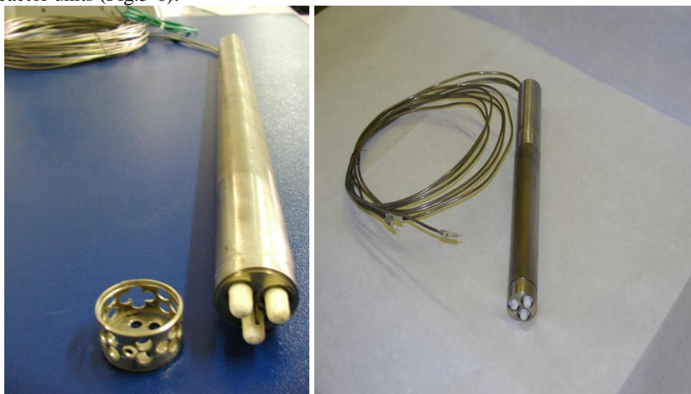
Figure 5 – The sensor with three sensitive elements for continuous oxygen monitoring, designed for advanced reactors.
