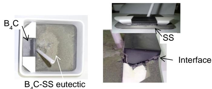
FIG. 14. Post-test observation in Case 2014-3.
