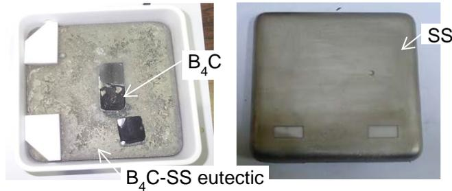
FIG. 10. Post-test observation in Case 2014-1.
