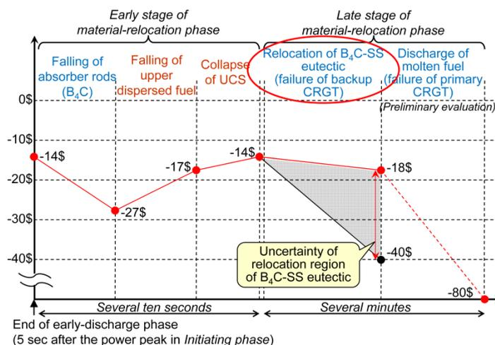
FIG. 1. Reactivity history in material relocation phase by exact perturbation calculation.
