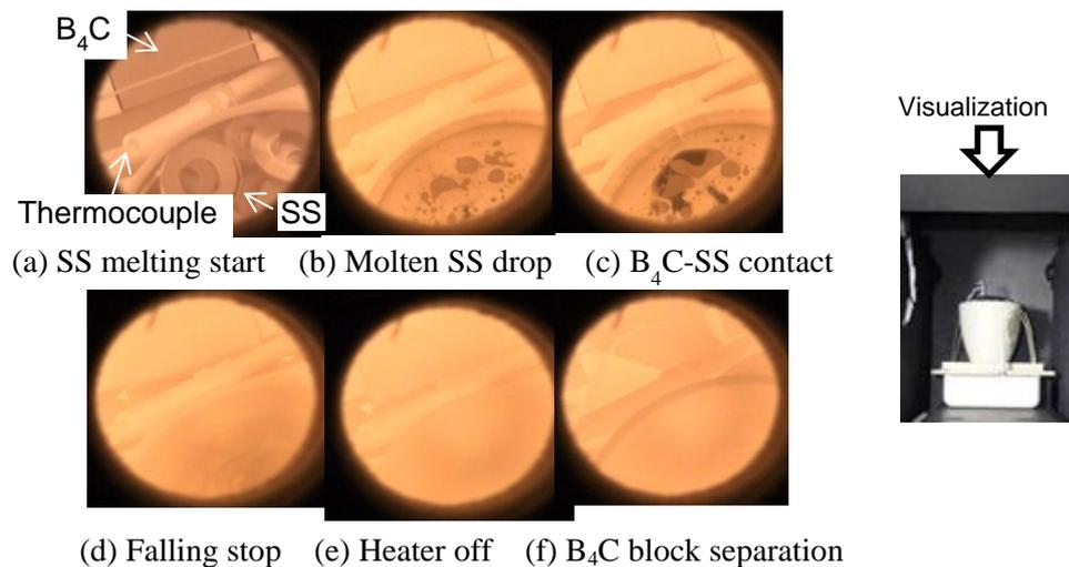
FIG. 8. Visualization of  $B_4C$ -SS eutectic reaction in Test 2014-1.
