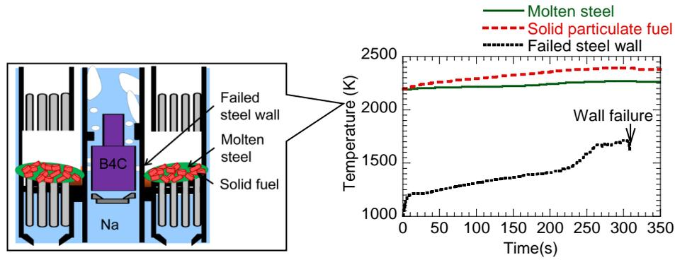
FIG. 2. Temperatures in a representative fuel assembly surrounding a control rod guide tube.
