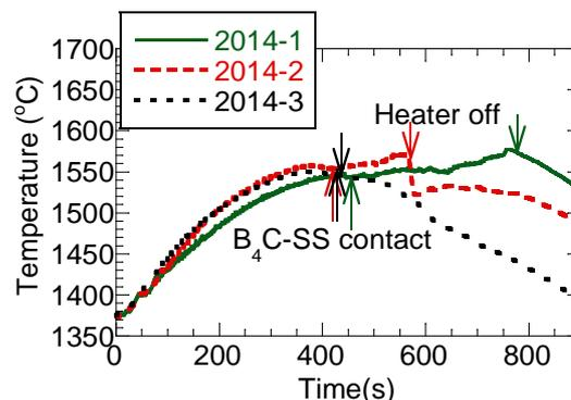
FIG. 9. Temperatures at  $B_4C$  block surface. (arrow colors correspond to test cases).
