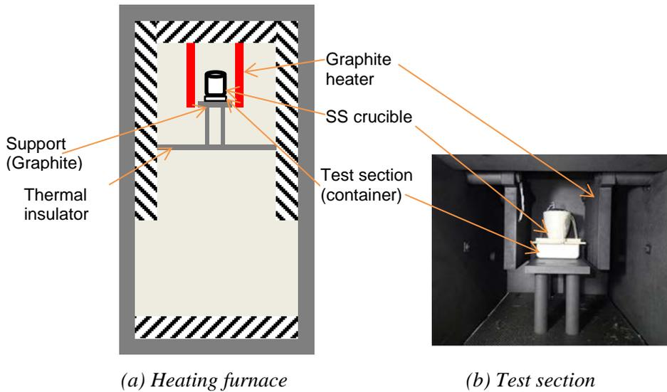
FIG. 4. Experimental apparatus.
