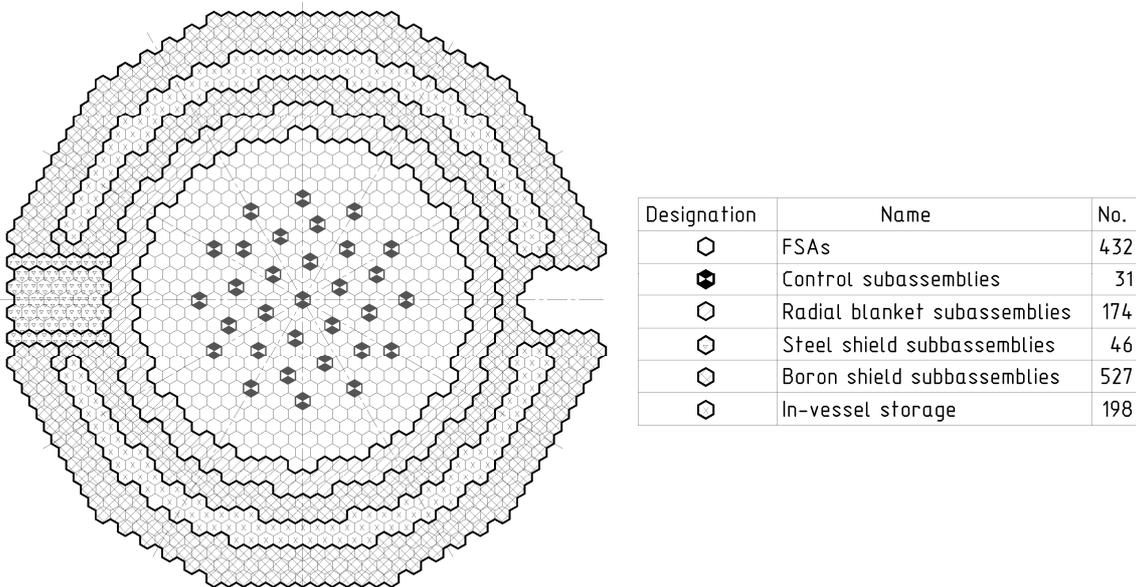
Figure 3: MOX fuel core layout
