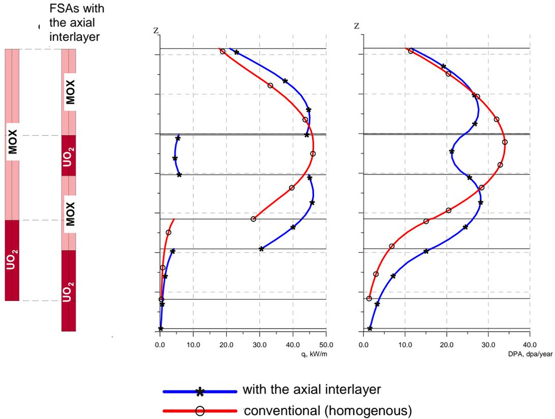
Figure 2: Axial distribution of the fuel pin linear heat rate and damage dose
