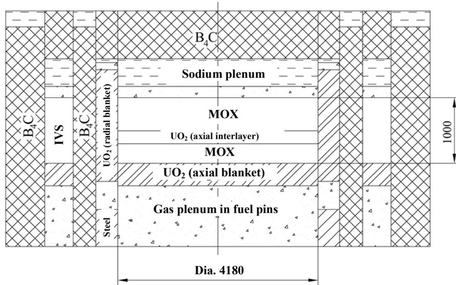
Figure 1: MOX-fuel core with the axial interlayer configuration
