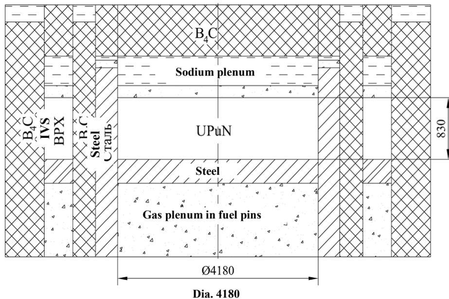
Figure 4: Nitride fuel core configuration
