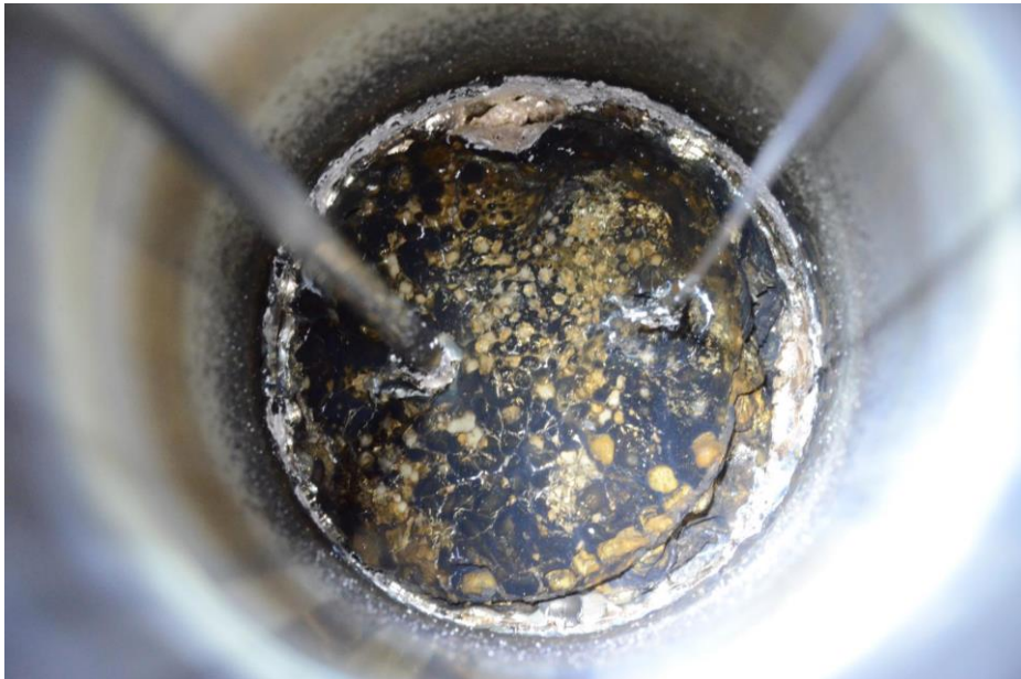
FIG. 9. Typical Sodium-CO 2 Solid Reaction Products Inside of Sodium-CO 2 Reaction Vessel Observed in SNAKE Experiments Conducted at Lower Temperatures.
