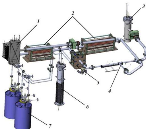
1 – sodium-air heat exchanger; 2 – electromagnetic pumps; 3 – heater; 4 – experimental model; 5 – electromagnetic pump-throttle; 6 – cold trap; 7 – sodium storage tanks
