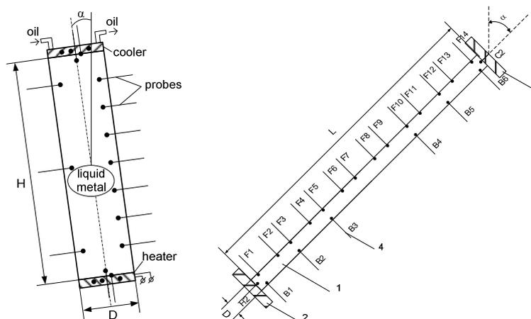
FIG. 2 – Schemes of experimental models to study free turbulent convection with aspect ratios  $l/d=5$  (left) and  $l/d=20$  (right)
