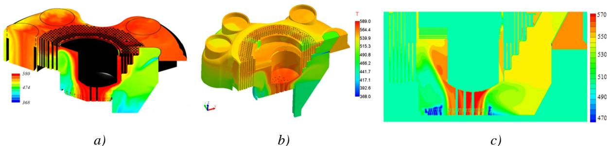
FIG. 8 – Results of simulation of the BN-600 reactor upper chamber. Temperature distribution ( $^{\circ}\text{C}$ ):
