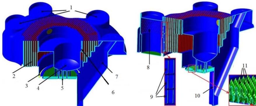
1 – intermediate heat exchanger; 2 – safety rods; 3 – annular gap around the support;
