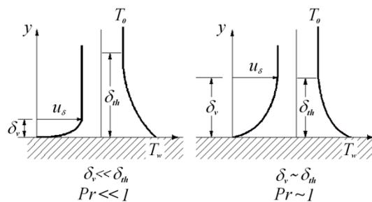
FIG. 1 – Effect of the molecular Prandtl number on relative thickness of the thermal boundary layer ( $u_s$ ,  $T_o$  – flow velocity and temperature respectively,  $T_w$  – wall temperature)
