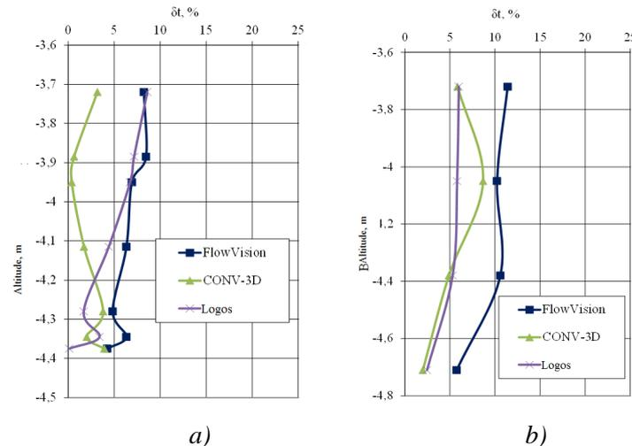
FIG. 9 – The relative deviation of calculated temperature values from measured values along the height of intermediate heat exchanger (IHX): a) 5 IHX-A, b) 4 IHX-B
