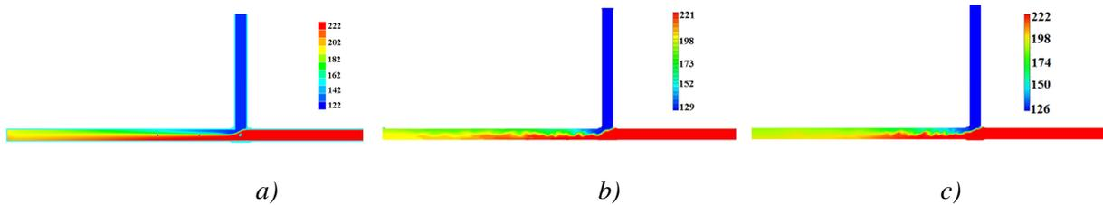
FIG. 5 – Coolant temperature distribution ( $^{\circ}\text{C}$ ): a) FlowVision, b) CONV-3D, c) LOGOS
