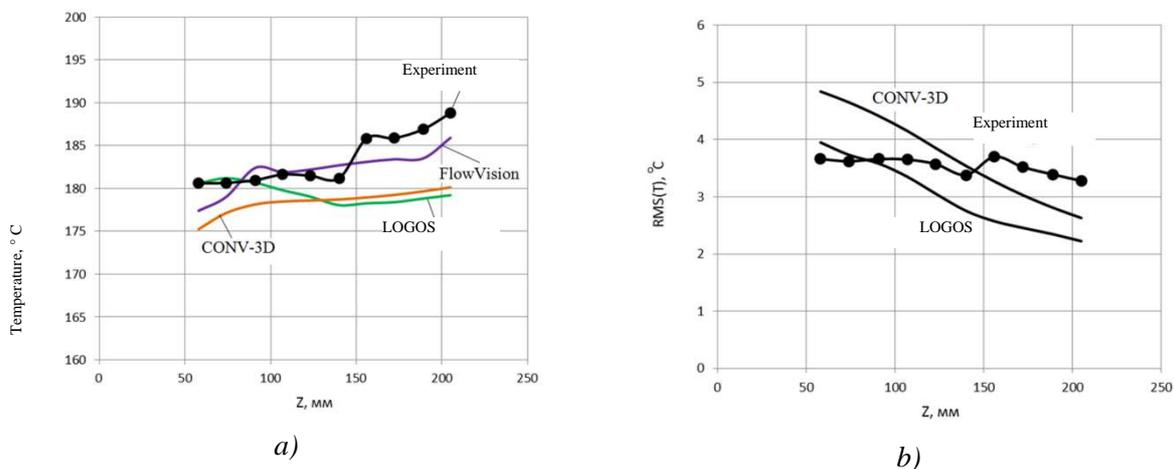
FIG. 6 – Comparison of the calculated results: a) average temperature dependence on coordinate  $Z$ ;
