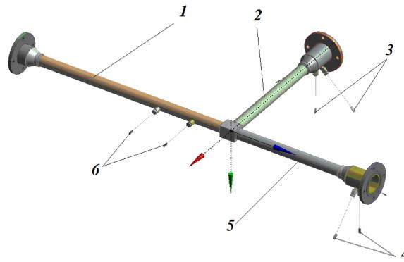
1 – mixing portion; 2 – “cold” sodium inlet portion; 3 – thermal couples at the “cold” branch inlet;
