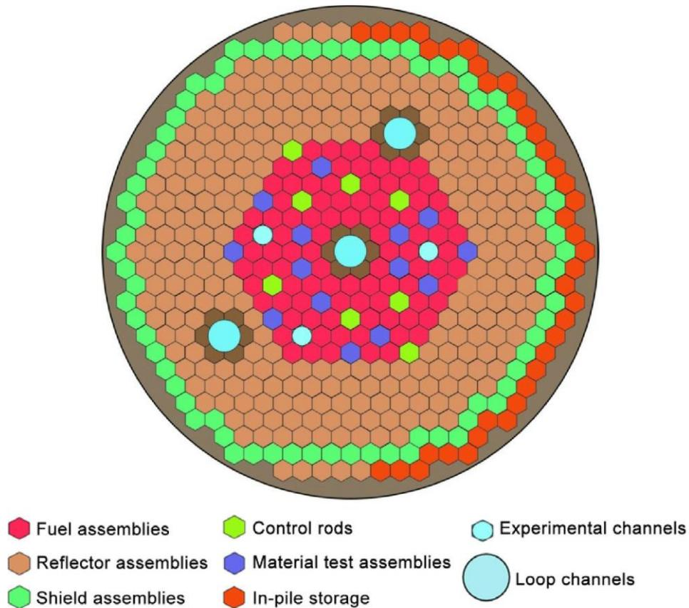
Fig. 4. Layout of MBIR reactor core
