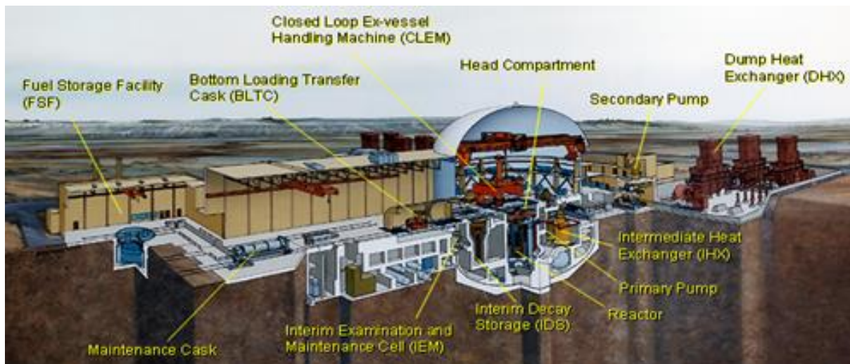
FIG. 2. FFTF Reactor Plant
