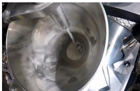
FIG. 2. Corkscrew-shaped powder agitator
