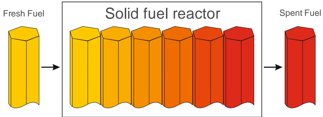
FIG. 1 Illustration of fuel burn-up distribution in the case of a solid fuel reactor.
