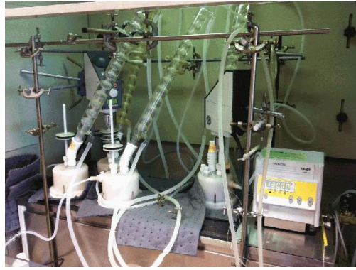
FIG.3. EDF R&D device for tests in aqueous sodium hydroxide
