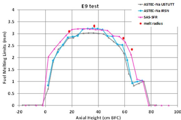
FIG. 3: CABRI E9 test: fuel melting limits
