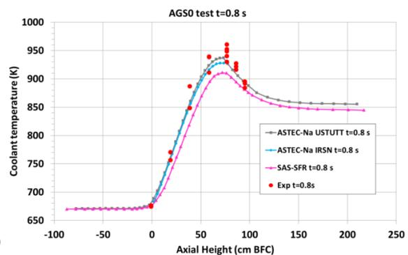
FIG. 4: CABRI AGS0 test: coolant temperature
