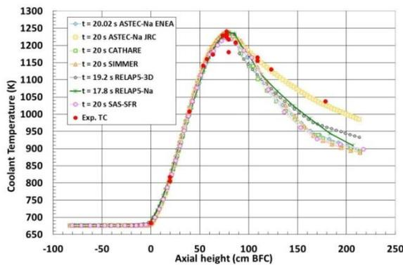
FIG. 1: CABRI BI1 test: Sodium temperature just before boiling onset around  $t = 20$  s
