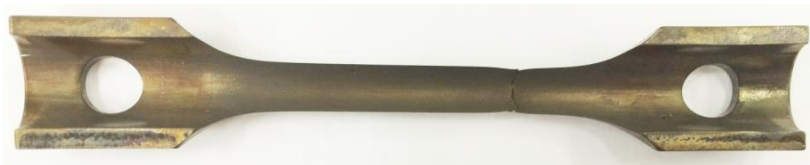
FIG. 4. A segment-type specimen machined from SG tubing after SSRT-testing in superheated steam at 505 °C
