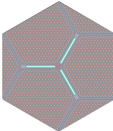
FIG.4. Cross-sectional view of the RBWR-TR unit cell, as modeled in MocDown and Serpent.
