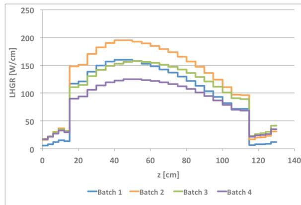
FIG.6.2 LHGR distribution for each of the four batches and the peak assembly value at EOC.
