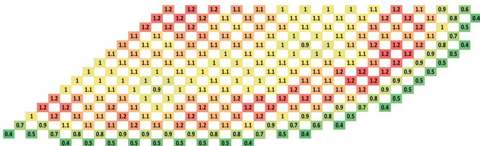
FIG.7.1 Power map for the RBWR-TR using FeCrAl cladding of 0.05 cm at BOC.
