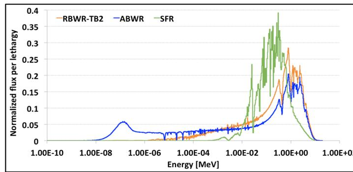
FIG. 1. Flux spectra in the RBWRs against an ABWR and an SFR.
