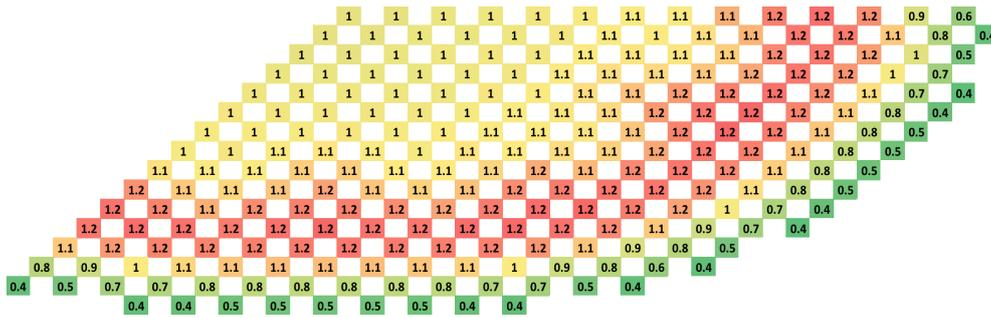
FIG.7.2 Power map for the RBWR-TR core using FeCrAl cladding of 0.05 cm at EOC.
