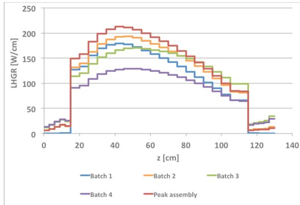
FIG.6.1 LHGR distribution for each of the four batches and the peak assembly value at BOC.
