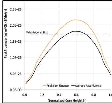
FIG.3. Fast fluences for the RBWR-TR design and the acceptable limits for Zircaloy-2.
