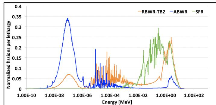
FIG. 2. Spectra of neutrons inducing fission in the RBWRs and other reactors.
