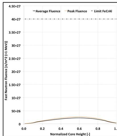
FIG.5. Fast fluences for the RBWR-TR design and the acceptable limits for FeCrAl.
