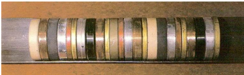
FIG. 3. Example of a pellet loading within a BFS tube (taken from [3])
