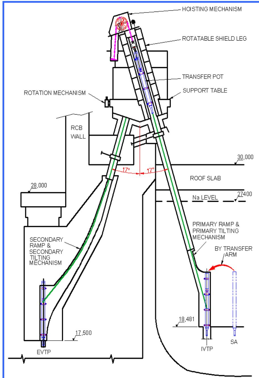
Fig. 4: Inclined fuel transfer machine
