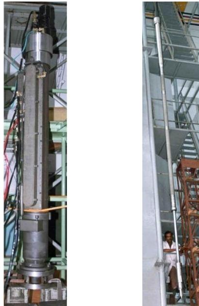
*Fig. 1. Upper and lower parts of Control & Safety Rod Drive Mechanism*
