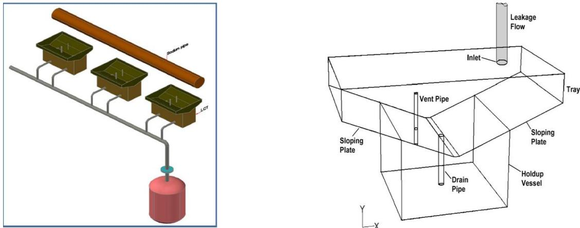
*Fig. 6: Configuration of Leak Collection Tray*
