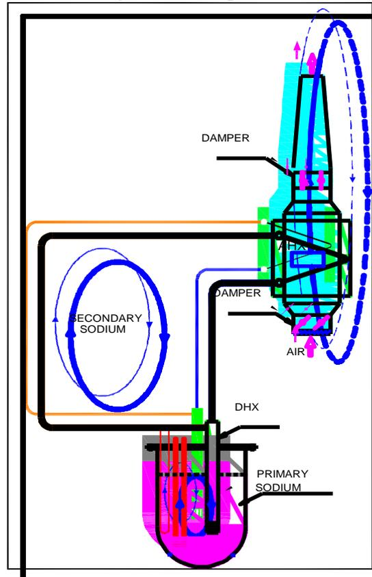
Fig. 2: Schematic of passive decay heat removal system for experimental studies
