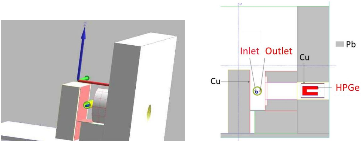
FIG. 4. Geometrical model of the measurement system (left: 3D view; right: cross-section view).
