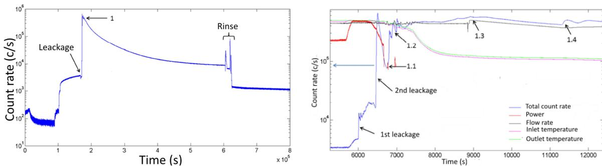
FIG. 6. Total gamma count rate as a function of time during the clad failure. Left: global profile; right: focus on the leakage.
