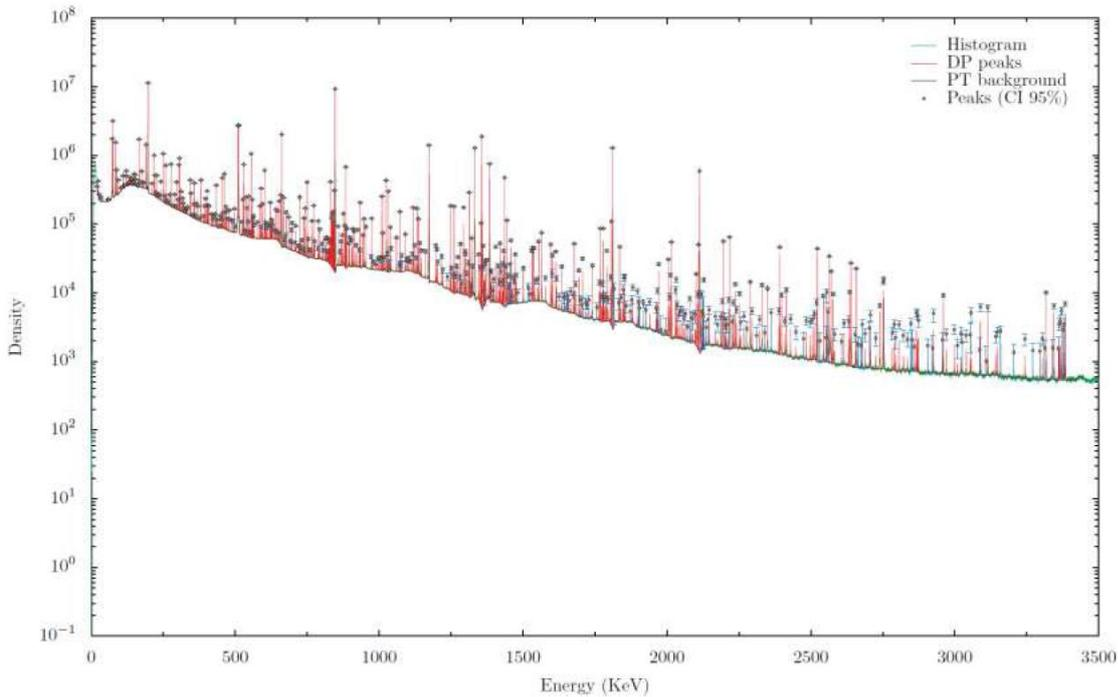
FIG. 6. Spectrum obtained during water coolant measurement after a clad failure.
