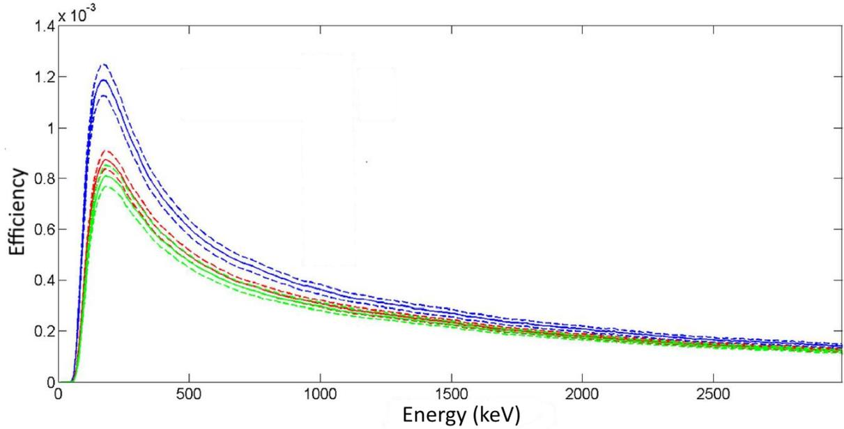
FIG. 5. Detection efficiencies for the inlet circuit (green) and for the outlet circuit (blue). Dash lines are  $1\sigma$  uncertainties.
