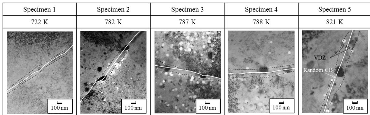
FIG. 1. TEM images; void distributions near random grain boundaries in the neutron-irradiated PNC316 steel specimens.
