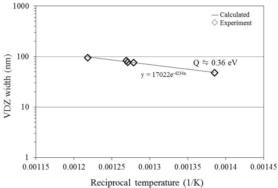
FIG. 2. Relationship between the VDZ width and reciprocal temperature.
