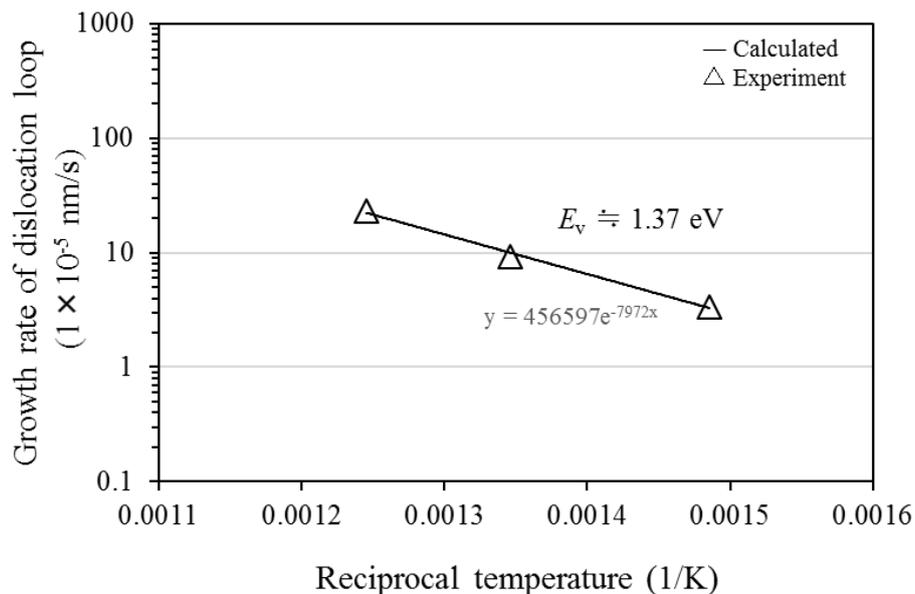
FIG. 3. Relationship between the growth rate of dislocation loop and reciprocal temperature.
