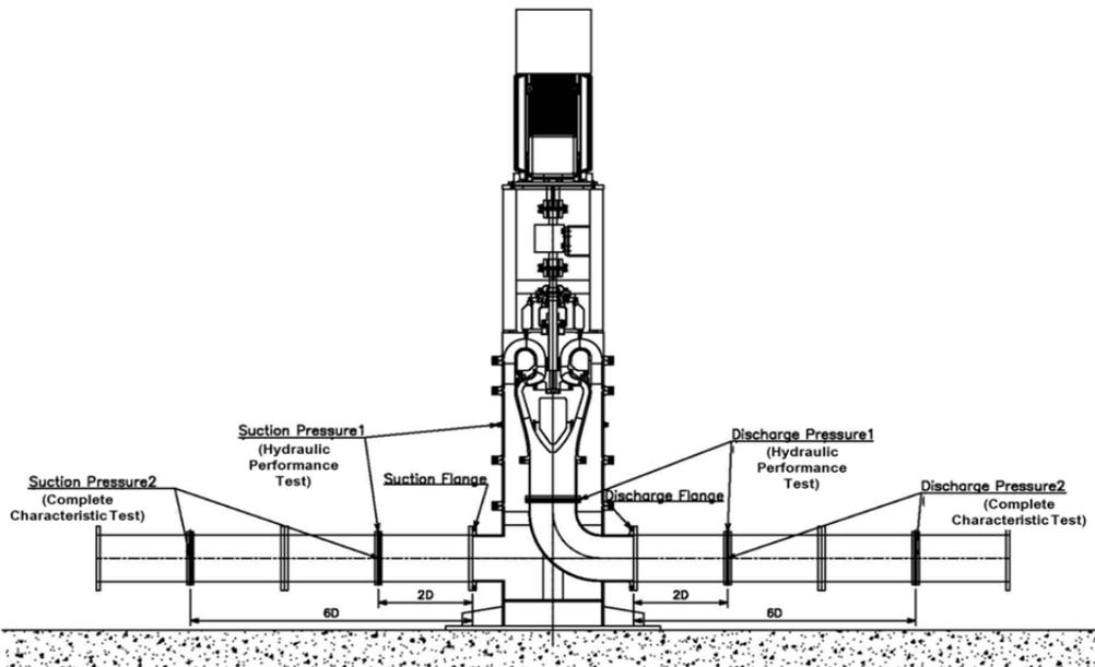
FIG. 3. The hydraulic test loop configuration for the model pump.
