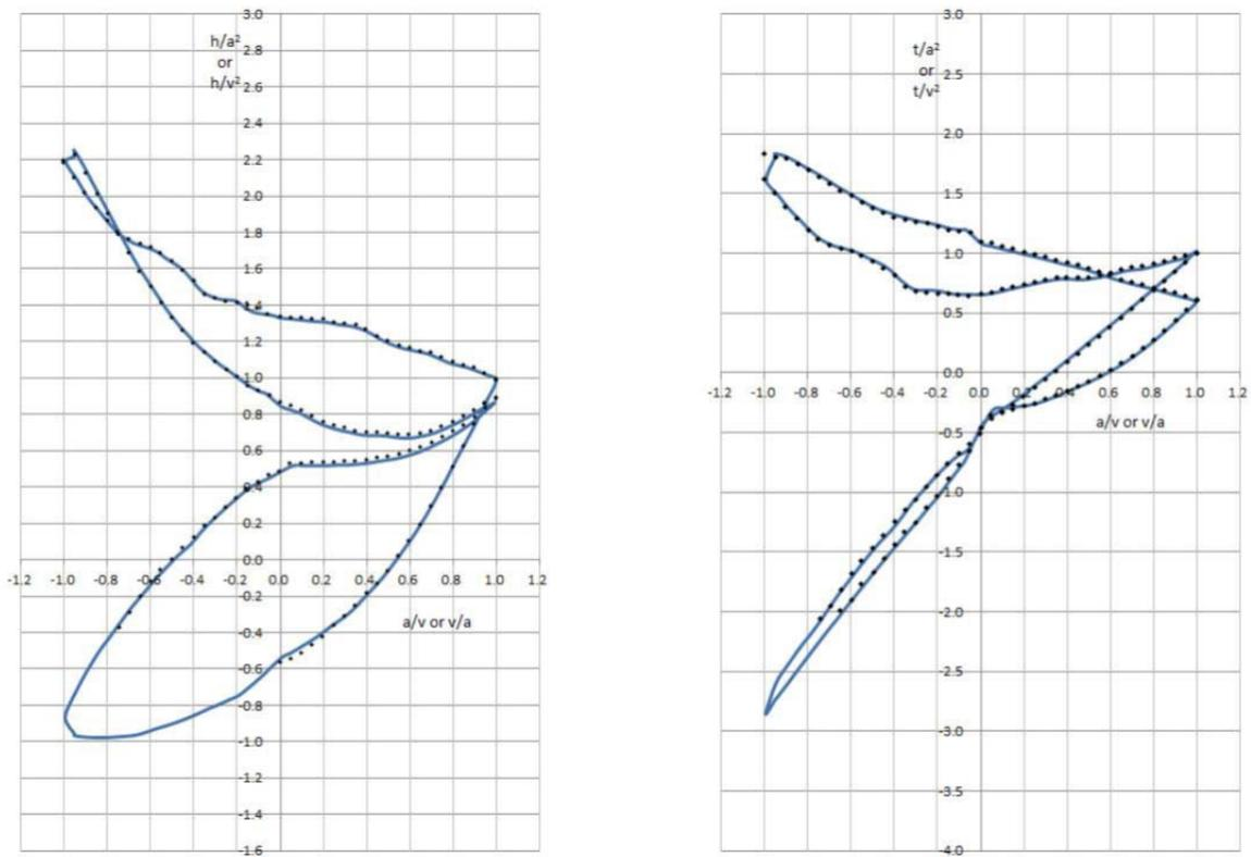
FIG. 7. The homologous head curve(left) and homologous torque curve(right), (solid line: 70% speed, dotted line: 100% speed).
