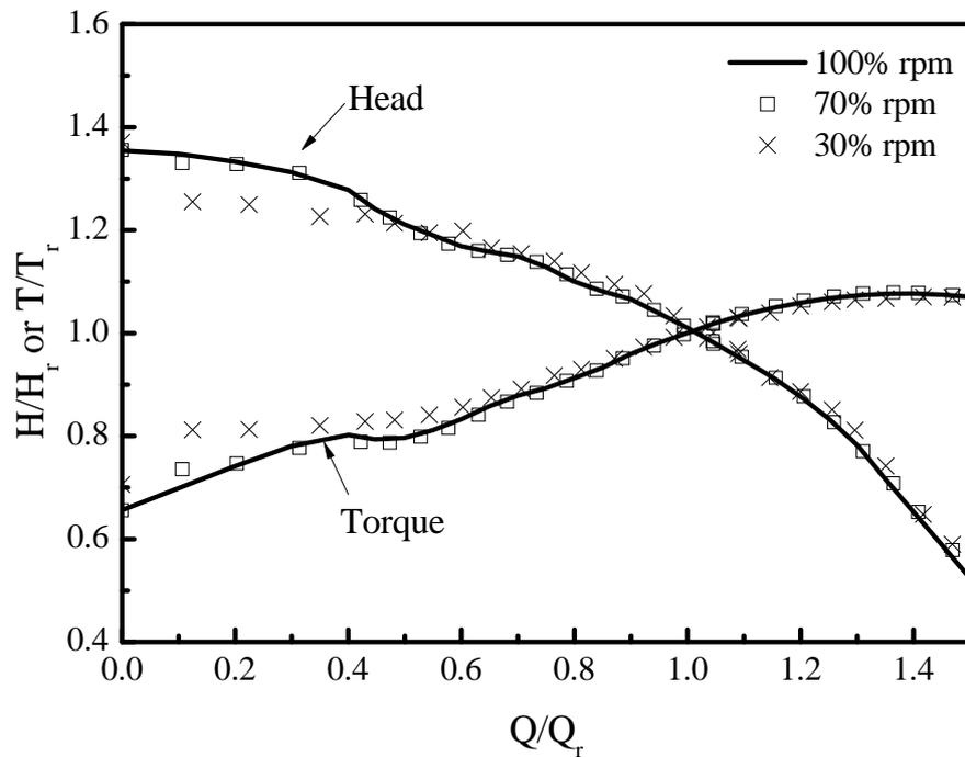
FIG. 5. The normalized flowrate-head and flowrate-Torque curve at 100%, 70% and 30% rpm conditions.
