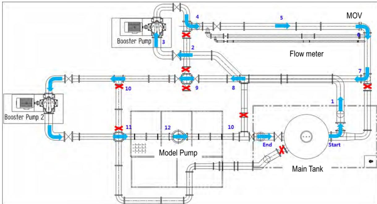
FIG. 1. The hydraulic test loop configuration for the model pump.
