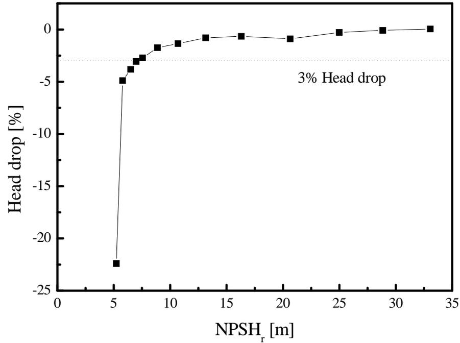
FIG. 6. The NPSH<sub>r</sub> curve of the prototype pump.
