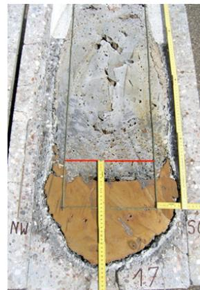
FIG. 8. Cross section of MOCKA crucible at KIT [8]
