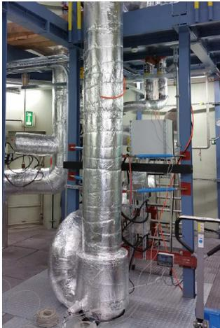
FIG. 3. KASOLA facility to study sodium transitional flow
