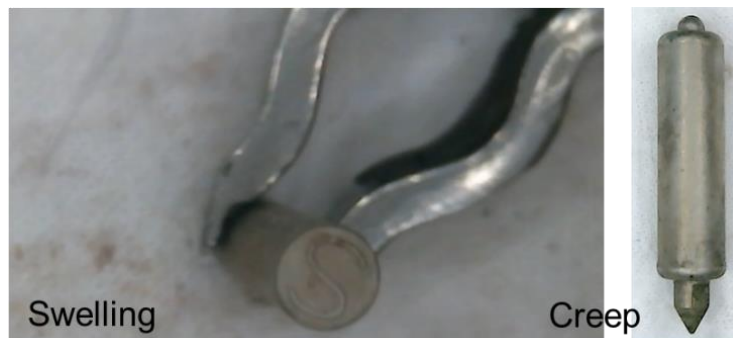
FIG. 8. Visual inspection of FC92 specimen after the interim inspection
