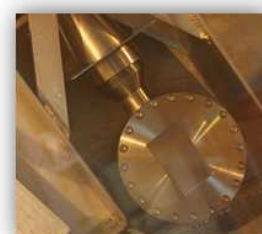
2014-15, 8 element phased array, tested in liquid sodium.
