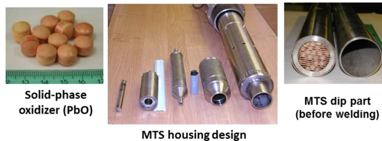
Figure 6 – Mass-transfer systems to implement the solid-phase method for HLMC oxygen potential control
