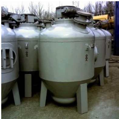
Figure 1. An example of a montejus loading system (with montejus preparation at the factory).
