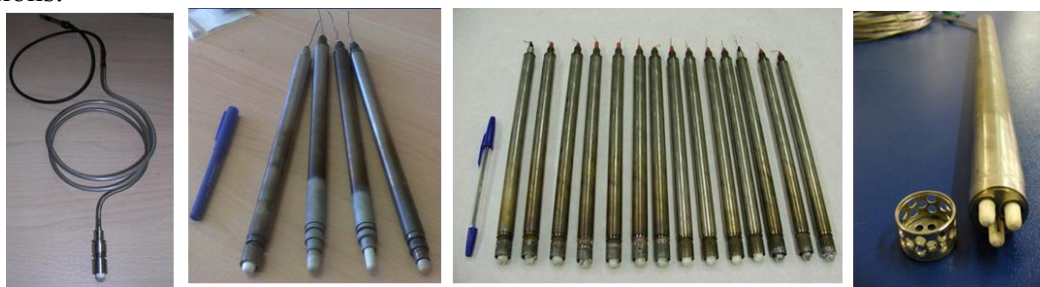
Figure 5 – Capsule-type oxygen thermodynamic activity sensors
