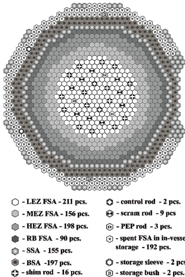
Figure 1 The full MOX fuel core layout
