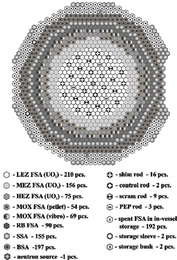
Figure 3. – The core layout for the fourth operation interval
