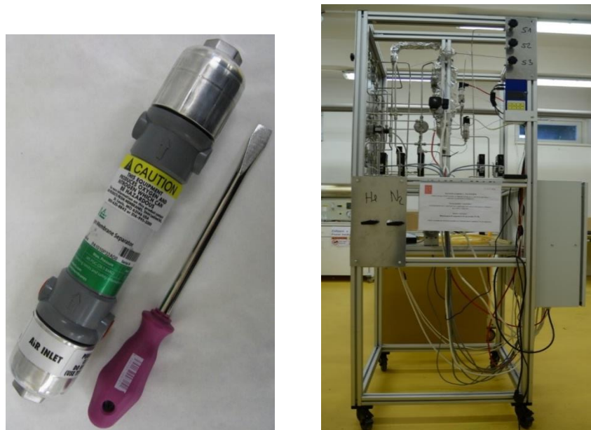
FIG. 3. Membrane module PRISM ® used for tests in the testing device.
