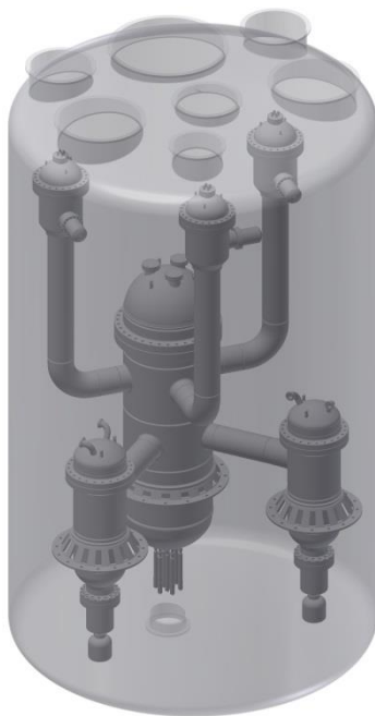
FIG. 1. ALLEGRO primary circuits with the decay heat removal system inside the guard vessel including its main parameters (concrete structures are not shown for simplicity).
